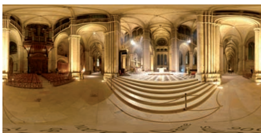
Figure 8: Equirectangular projection of the image in figure 7. Equirectangular is the most commonly used projection to display full spherical panoramas. The floor occupies a large area, but the ceiling is compressed. Image ©S. Pérez-Duarte
