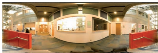
Figure 1: Lambert Cylindrical Equal Area. The poles are compressed and the emphasis is in the area in the middle. Compare this image to figure 5; the tripod used to take these photos is not recognizable. Image ©D.M. German
