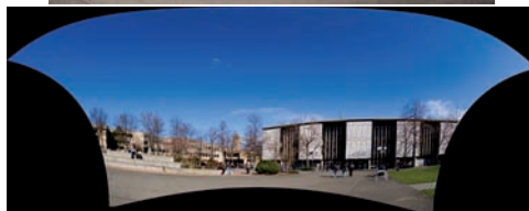
Figure 12: Automatically remapping an image from a Fish-eye lens to Lambert Equal Area (the original is above).
