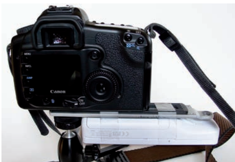
Figure 9: The Wii Remote mounted under a Canon 20d camera using the tripod socket.
