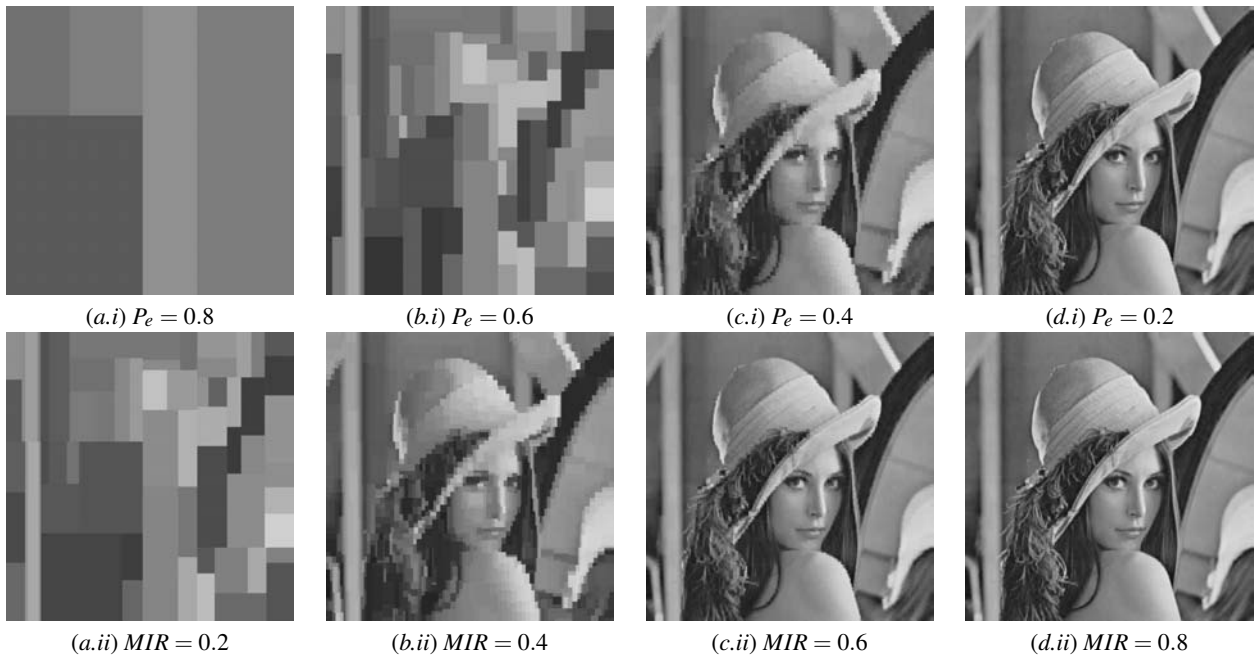
Figure 3: Lena image with luminance Y_{709} for different values of P_e (i) and MIR (ii). The (RMSE, PSNR) values for (i) are (45.47, 14.66), (30.02, 18.27), (14.03, 24.88), and (8.21, 29.54), respectively. For (ii) we have (32.98, 17.45), (16.23, 23.61), (9.71, 28.07), and (6.25, 31.90), respectively.
