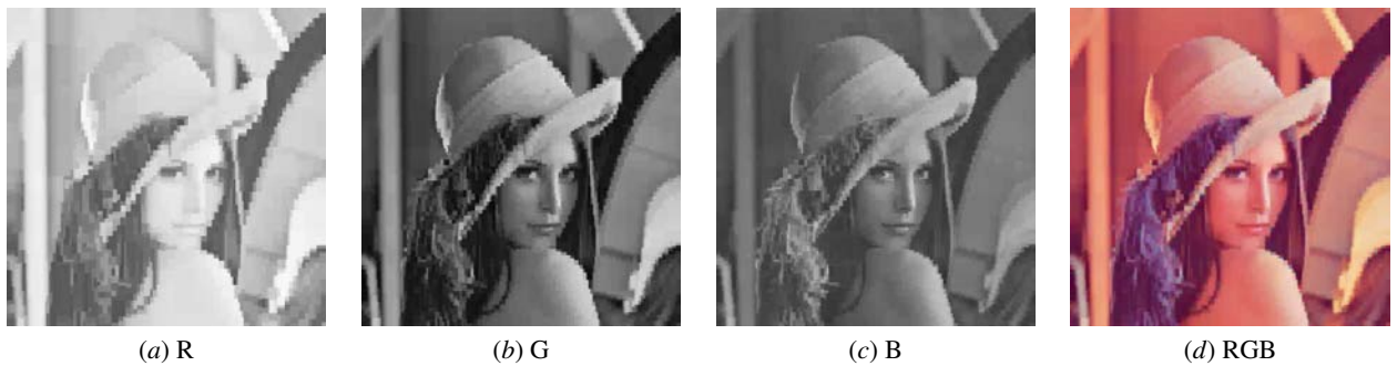
Figure 4: Lena image in RGB system with P_e = 0.4 . We obtain (a) 1835 ( r = 0.70 ), (b) 3692 ( r = 1.41 ), and (c) 4179 ( r = 1.57 ) regions. The merging image (d) has RMSE=13.20 and PSNR=25.32.
