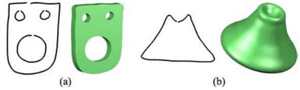
Figure 6: Sketched 2D curves can also be used to create (a) linear sweeps and (b) surfaces of revolution.
