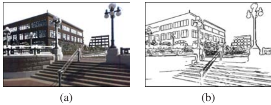
Figure 1: (a) Data deficiency is apparent in an attempted photorealistic rendering of outdoor scanned data. (b) It is less noticeable in a sketch rendering of the same data.
