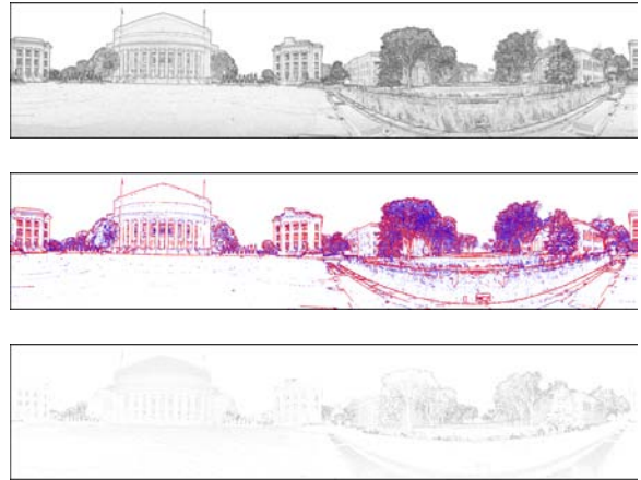
Figure 2: Feature extraction of a panoramic scan. From top to bottom: gray-scale-encoded feature degrees, feature points (red: directional points; blue: non-directional points), and dithering points.
