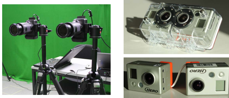
Figure 7.8: The setups used in our experiments. From left to right: A pair of Canon EOS 550D cameras; the GoPro 3D Hero system.
