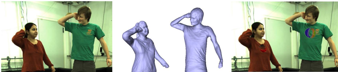
Figure 8.6: One of our performance capture results. Left to right: input video, reconstructed geometry, edited video with virtual logo added.
