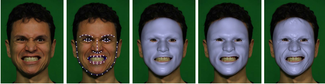
Figure 9.5: Algorithm overview: Left to right: (a) Input video frame, (b) sparse feature tracking, (c) expression and pose estimation using a blend shape model, (d) dense expression and pose correction, (e) shape refinement.
