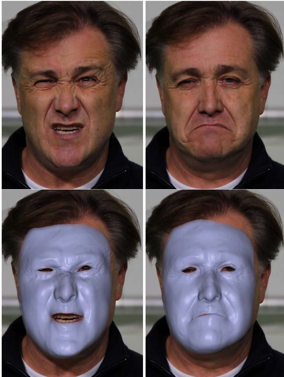
Figure 9.7: Monocular facial performance capture results for very expressive and fast facial gestures and challenging head motion for up to 1000 frames.
