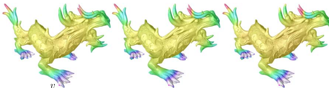
Figure 6.1: The vibration distance on the Chinese dragon model in various resolutions: 10k, 50k, and 130k vertices. Distance to vertex v in continuous coloring: from white being similar to red being dissimilar. Results are visually close indicating that distances can be well-approximated on coarse meshes.
