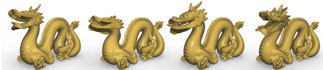
Figure 3.1: Reduced simulation of a geometrically nonlinear deformable object with 92k tetrahedra computed at over 120Hz after about four minutes of preprocessing (see Table 3.3).
