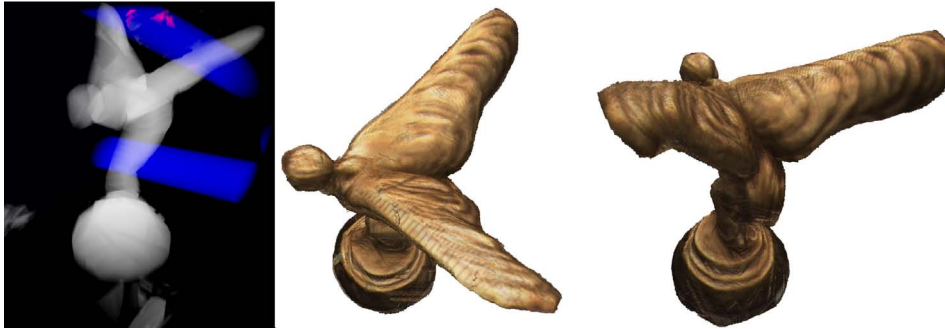
Figure 6.2: Semi-transparent mode (left): Visual-hull voxels are shown in white with a low density. Outside voxels covered by the brush are shown in blue. Finally, visual-hull voxels covered by the brush are shown in red. Image-based shading (middle and right): Pixels are transferred from the kaleidoscope image.
