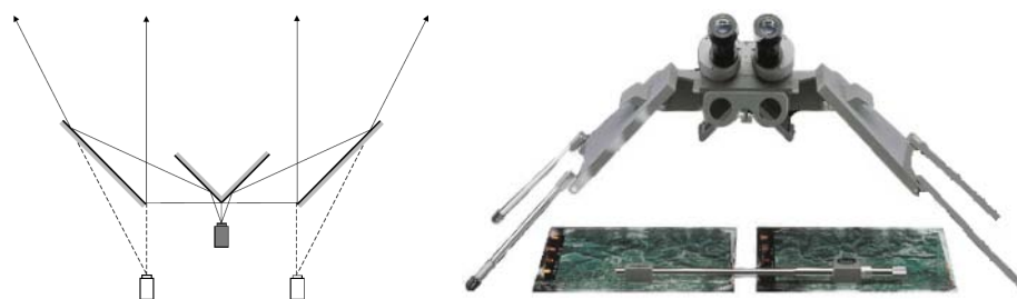
Figure 2.4: Design for a four mirror stereo camera or viewing device [Gluckman00] (left). The Sokkia MS27 commercial stereo viewer for aerial imagery (right).
