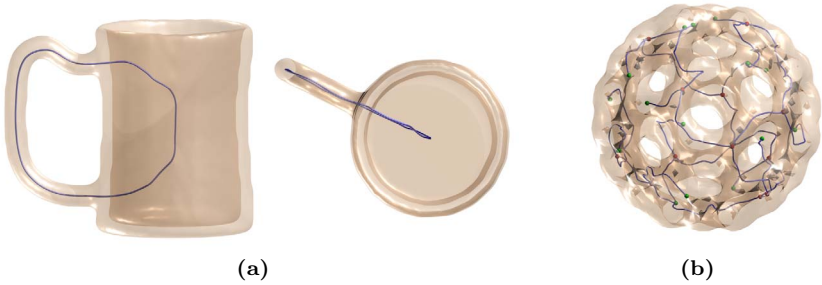
Figure 5.12: Two datasets where the naive method fails. A mug does not belong to the class of generalized cones and its deep cavity is not represented properly by the skeleton (a). The multi-view system employed by the algorithm is not able to provide an exhaustive representation of the complex morphology of the buckyball molecule (b).
