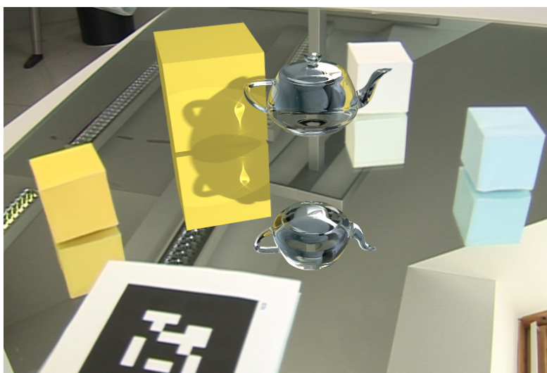
Figure 4.6: Caustics can be created by both virtual and real specular objects. The virtual glass teapot casts a caustic to the virtual diffuse cube. Part of this caustic was created by the reflection of light on the real mirror. The generated caustic is correctly reflected in the real mirror. Moreover, the real environment is refracted in the teapot.
