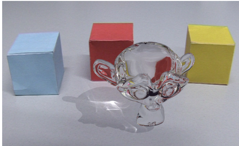
Figure 4.4: The resulting image produced by our AR rendering system. The image was rendered by shooting 9 rays per pixel to obtain a high-quality result and to reduce aliasing artifacts. 1M photons were shot in the photon shooting phase. The scene was rendered at 1fps, and the rendering rate can achieve 15 fps by decreasing the number of samples per pixel. There is one virtual glass monkey, casting caustics onto real objects, and three real cubes in the image.
