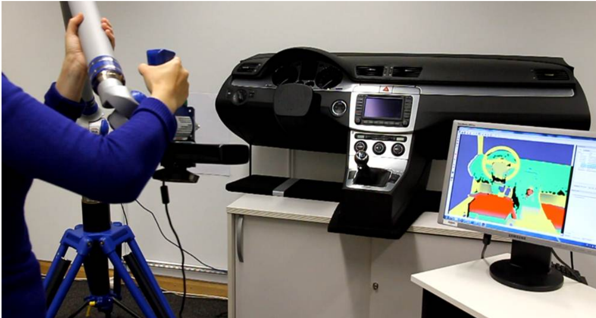
Figure 4.2.: 3D difference detection with a Kinect depth camera and an industrial measurement arm.
