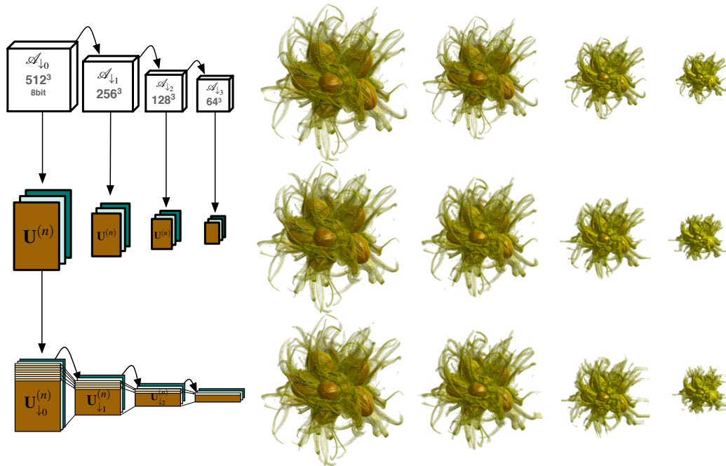
Figure 4.7: Factor matrix subsampling (bottom row) compared to direct TA (middle row) derived from original subsampled input datasets (top row). From [Suter et al., 2013].
