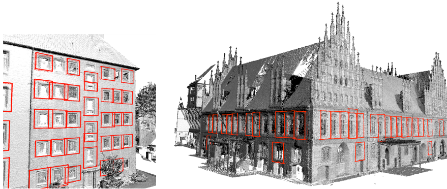
Figure 7.17: Further detection results for the big Hannover scene (see Figure 7.15). A considerable percentage of all windows is detected.
