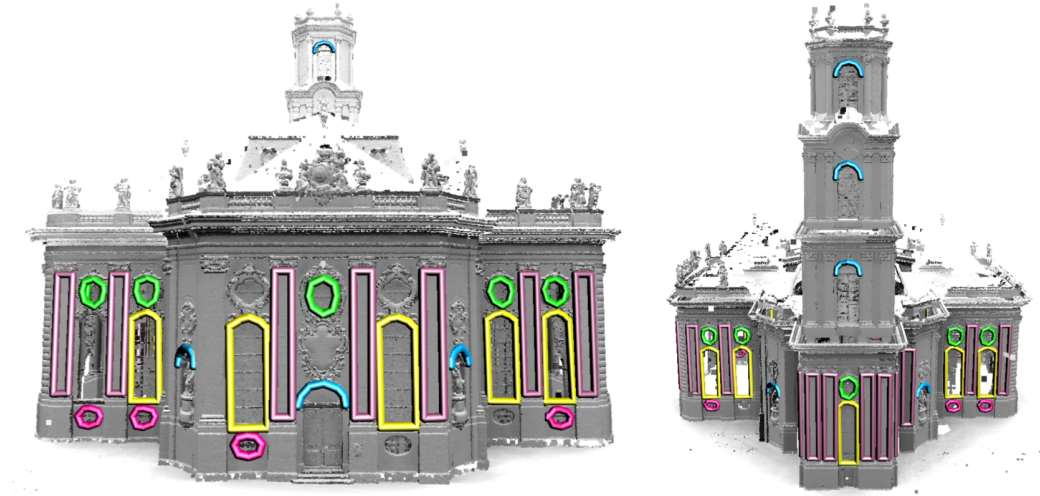
Figure 6.1: We propose an interactive learning algorithm for 3D object detection. Object classes can be intuitively defined with user strokes. In this example, 2-3 instances have been sketched on the model for each class (indicated by different colors). Further instances are found automatically using inference on a Markov chain model.
