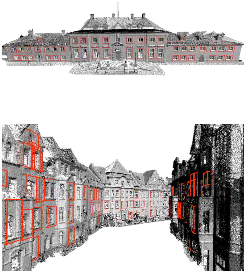
Figure 7.16: Detection results for the big Hannover scene (see Figure 7.15). The top shows the Wilhelm Busch museum which is part of the training region. The bottom shows detected windows in a street of houses in the test region.
