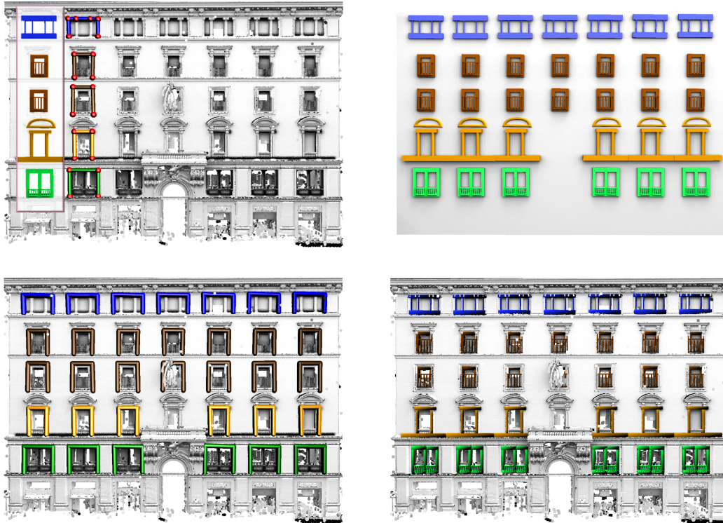
Figure 6.19: The detected object correspondences are used to align synthetic 3D models with detected objects of different (color coded) categories. The upper left shows the training examples and the matching primitives. The lower left shows all detected shapes. The right side shows the aligned primitives.
