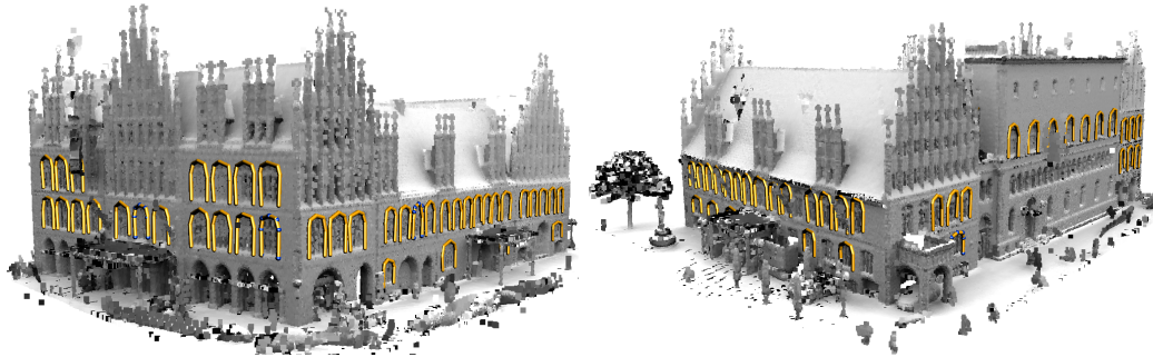
Figure 6.13: Single-class learning: Detecting “all windows”. Training data (windows with blue part positions) consists of 4 exemplar windows. Figure 6.12 shows a closeup of different window types detected by this class. In the example of Figure 6.8 these types have been trained individually.
