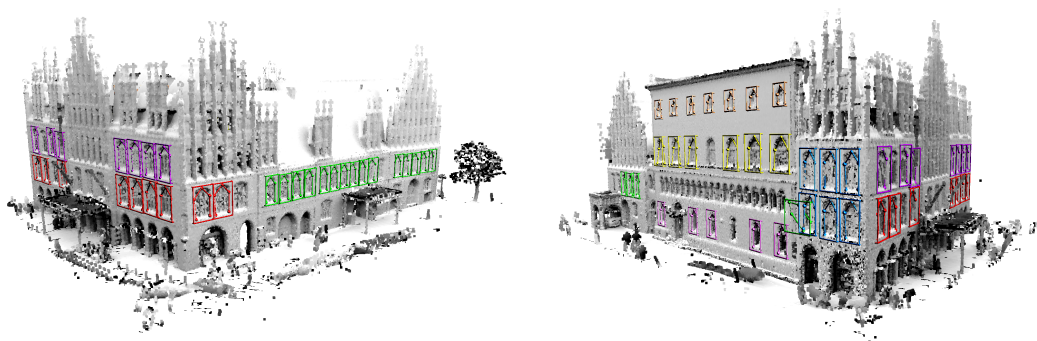
Figure 7.19: Multi-class learning results for the old town hall. Each class was trained with 3 exemplars.
