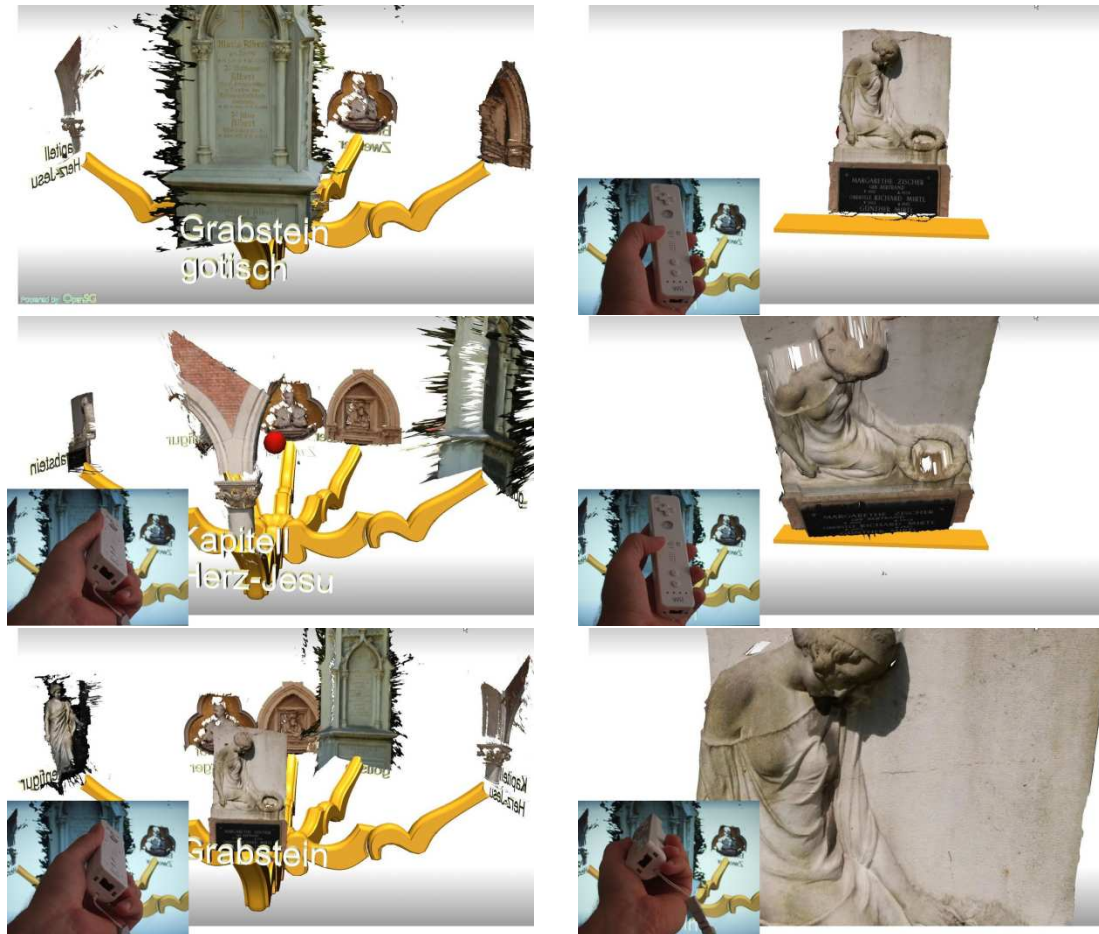
Fig. 5.9 Example of a 3D presentation. Left column top to bottom: The user can rotate the chandelier horizontally. Right column top to bottom: One object is chosen for inspection, and the user can orbit around it. – The objects shown are not high-quality artifacts but only examples.
