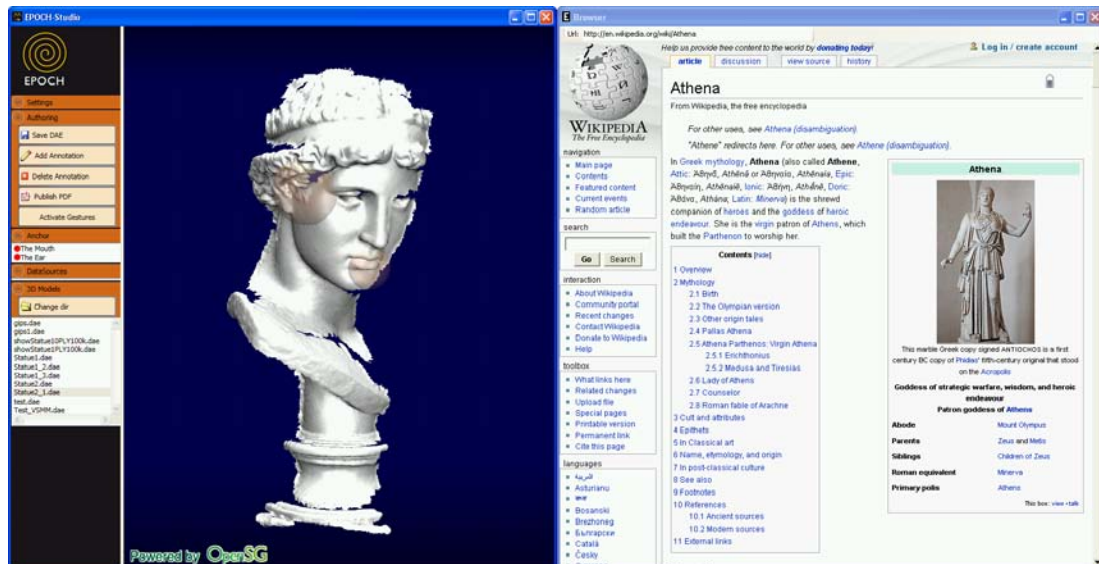
Fig. 3.16 The 3D model is annotated using the EpochStudio . The software is composed of a menu (left), a 3D view for the detailed inspection of the model (middle), and a browser for web-based research (right). Annotations can be placed on spots on the surface of the 3D model, shown as transparent balls. Annotations can be connected to one or multiple URLs.
