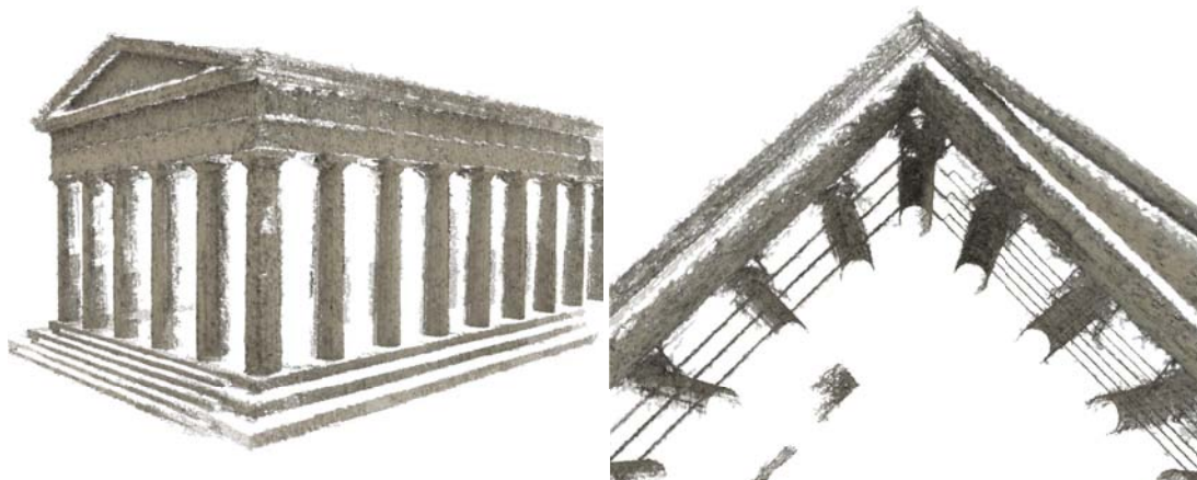
Fig. 2.10 The image-based 3D reconstruction of the Theseus temple for one sequence of photos. To reconstruct the whole temple, several photo sequences are necessary.
