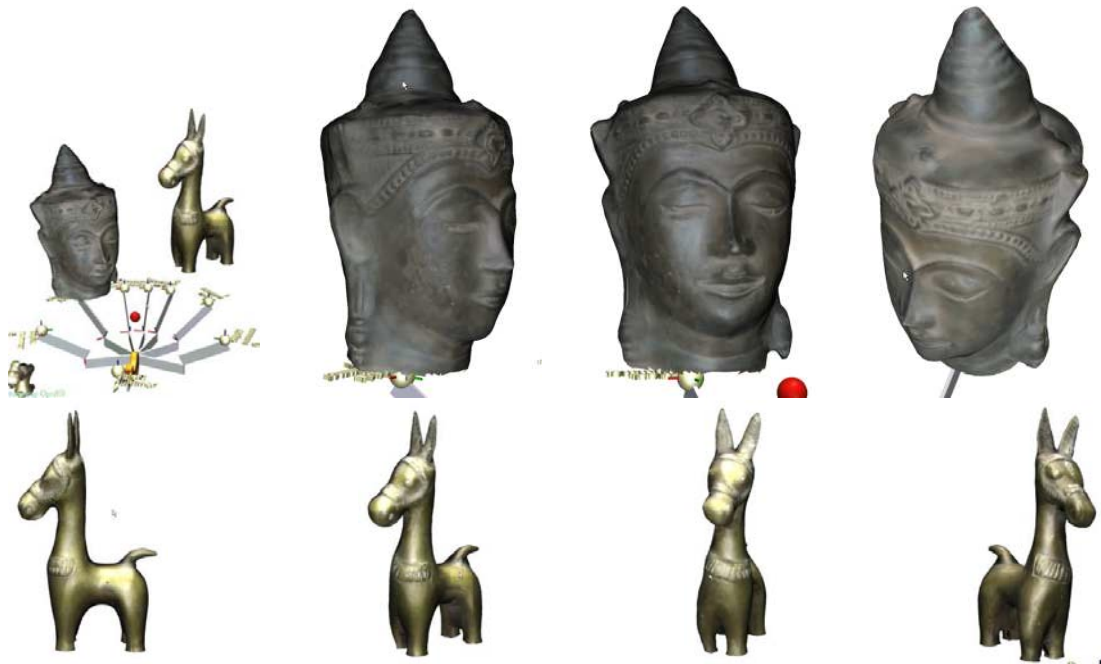
Fig. 5.11 Authoring a presentation with BTF-models. They are loaded and rendered using an OpenSG extension module that makes use of advanced vertex and pixel shaders. Models are courtesy Gero Müller and Reinhard Klein, Univ. Bonn, Germany
