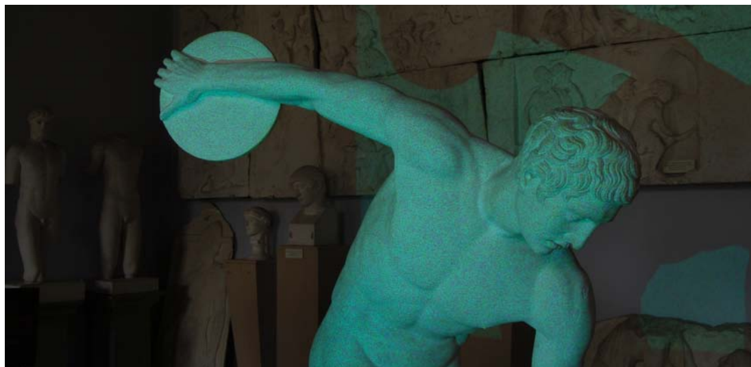
Fig. 2.11 This is one of the photos used for reconstruction. The projected random color pattern helps to identify feature points on the otherwise homogeneous surface.
