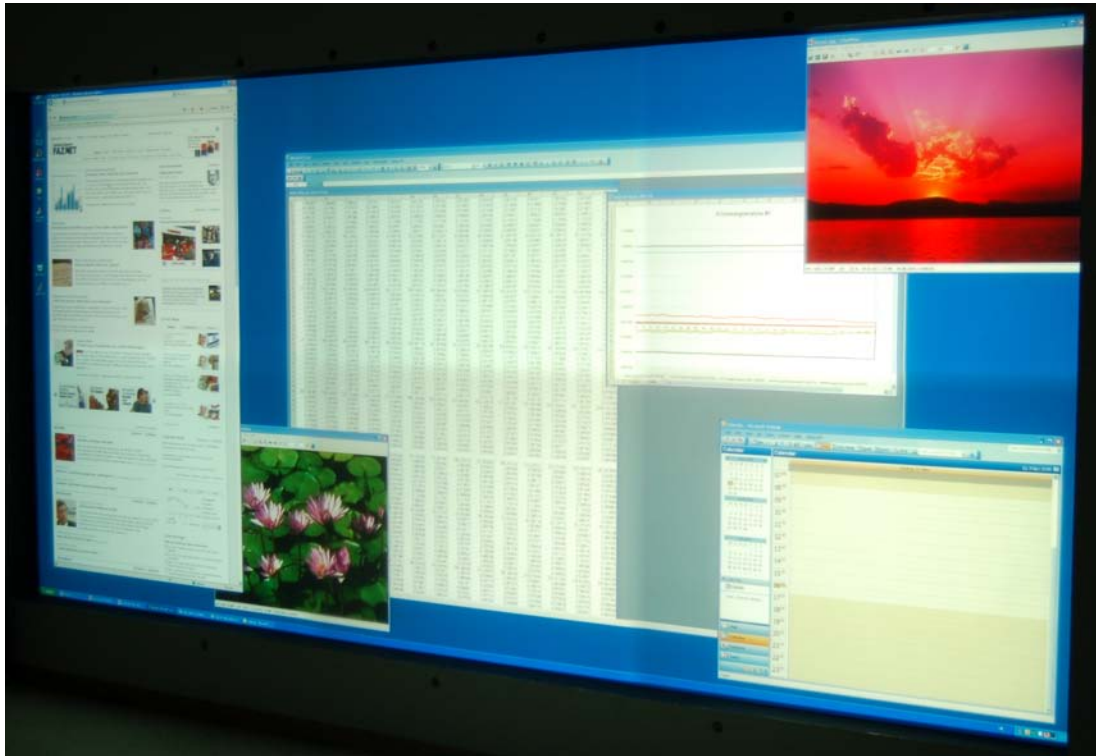
Fig. 4.48 Our tiled display with 3 \times 2 projectors has about 4000 \times 2000 pixels. The rendering is done on 3 PCs which are controlled by a master. Each render slave is connected to two projectors.
