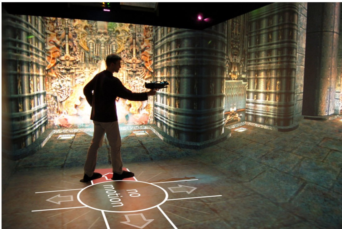
Fig. 4.35 The user's head position controls the walk navigation speed in the game Quake III Arena . In this image the user moves sideways by standing left to the center. His hands are free for other interaction devices such as the gun. The bottom marks are overlaid for illustration purposes and are not visualized within the game.
