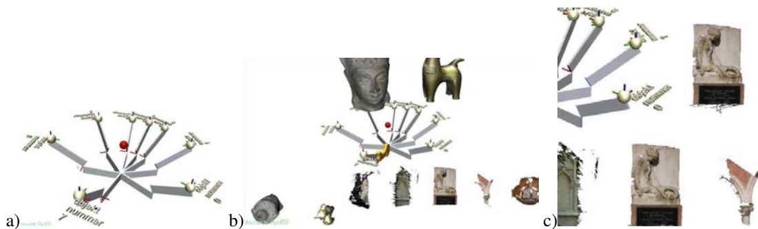
Fig. 5.14 Authoring via drag-and-drop. a) A blank layout consists of many drop targets. b) The “model bar” is filled via drag-and-drop from the file system with 3D models, 2D images, and 1D text strings. c) Objects are dragged interactively from the model bar to drop targets in the 3D scene, where they automatically align to the local coordinate frame.
