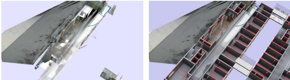
Fig. 5.24 Multiple video textures are added to the scene by duplicating the geometry. The left image shows the output of the video texture shaders which have discarded all pixels outside of the video image. In the right image the video textures are combined with the original scene geometry.
