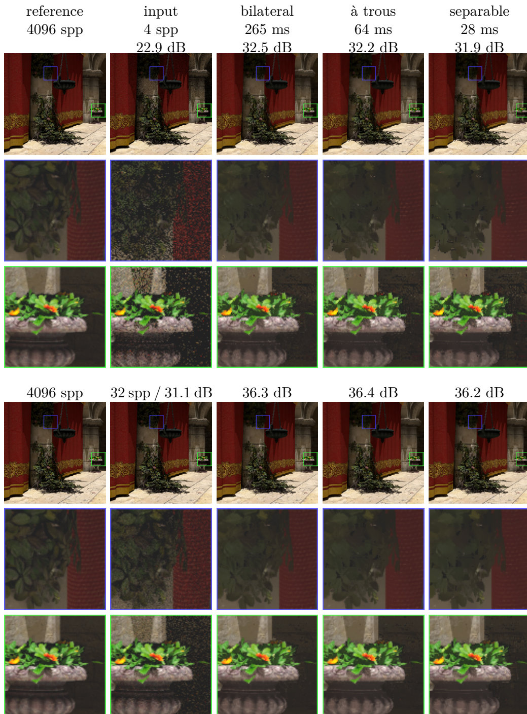
Figure 3.12: A comparison of filtering steps. “bilateral” is the cross bilateral filter used in the original algorithm, “à trous” is a variant of the À-Trous scheme [28], and “separable” is our variant of the separable bilateral filter [102]. Below the identifiers are the number of samples per pixel (spp), filtering time (in ms), and the PSNR (in dB). The blow-ups had their brightness increased for print.
