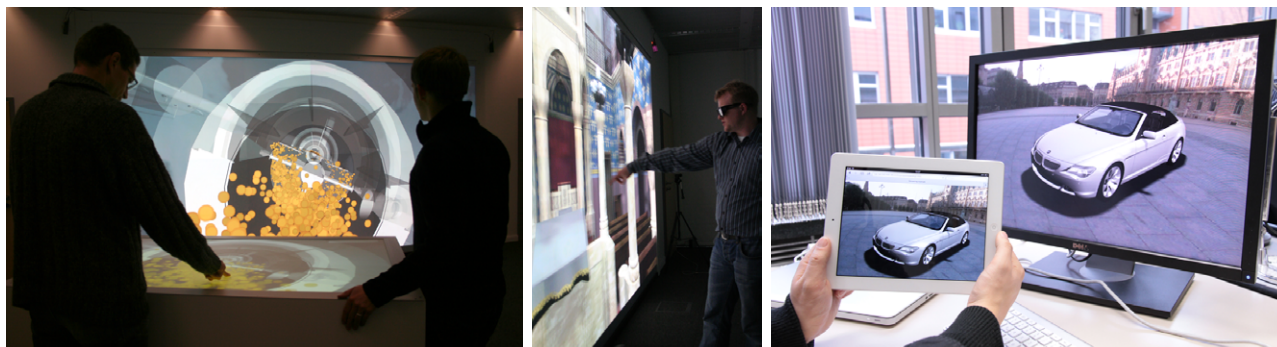
Figure 5.2: Some use cases. Left: an application running on a touch table and a large tiled display wall ( 6 \times 4 tiles, 8640 \times 4200 pixels). Middle: stereoscopic rendering on the same display wall. Right: video stream from desktop to web page, viewed in a browser on a tablet.
