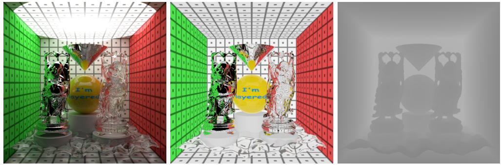
Figure 3.2: Left: a test scene containing reflecting/refracting surfaces. Middle: color range buffer generated by rendering with a single unoccluded head light and ambient light. It captures normals and textures (even in reflections/refractions). Right: depth range buffer containing geometric edges.
