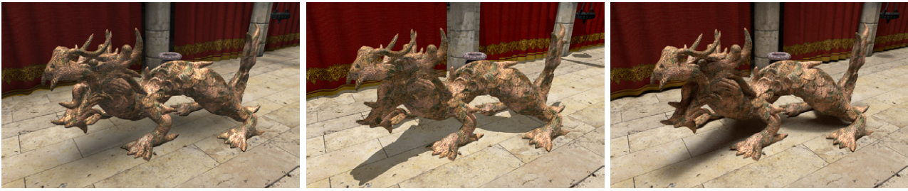
Figure 5.6: The same scene rendered with three different renderers by switching through viewports. Left to right: rasterization, whitted-style ray tracing, path tracing.
