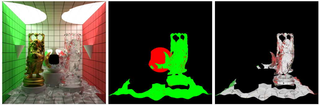
Figure 4.20: Left: the “Cornell specular 2” scene contains many reflecting/refracting surfaces. Middle: mask for the hybrid filter; pixels that are reflecting and refracting at the same time are green, pixels that are either reflecting or refracting are red. Pixel filtering is only applied to green pixels, radiance filtering to the rest. Right: range buffer for pixel filtering.
