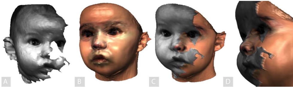
Figure 2.8: Example of the reconstruction of missing data by the use of a sample database of 3D scans. (A) Input: Incomplete 3D scan. (B) Best estimate from the the known database. (C) Merged scan and estimate. (D) Errors may occur, in particular at the boundaries, which need special treatment (such as smoothing) to appear more natural.
