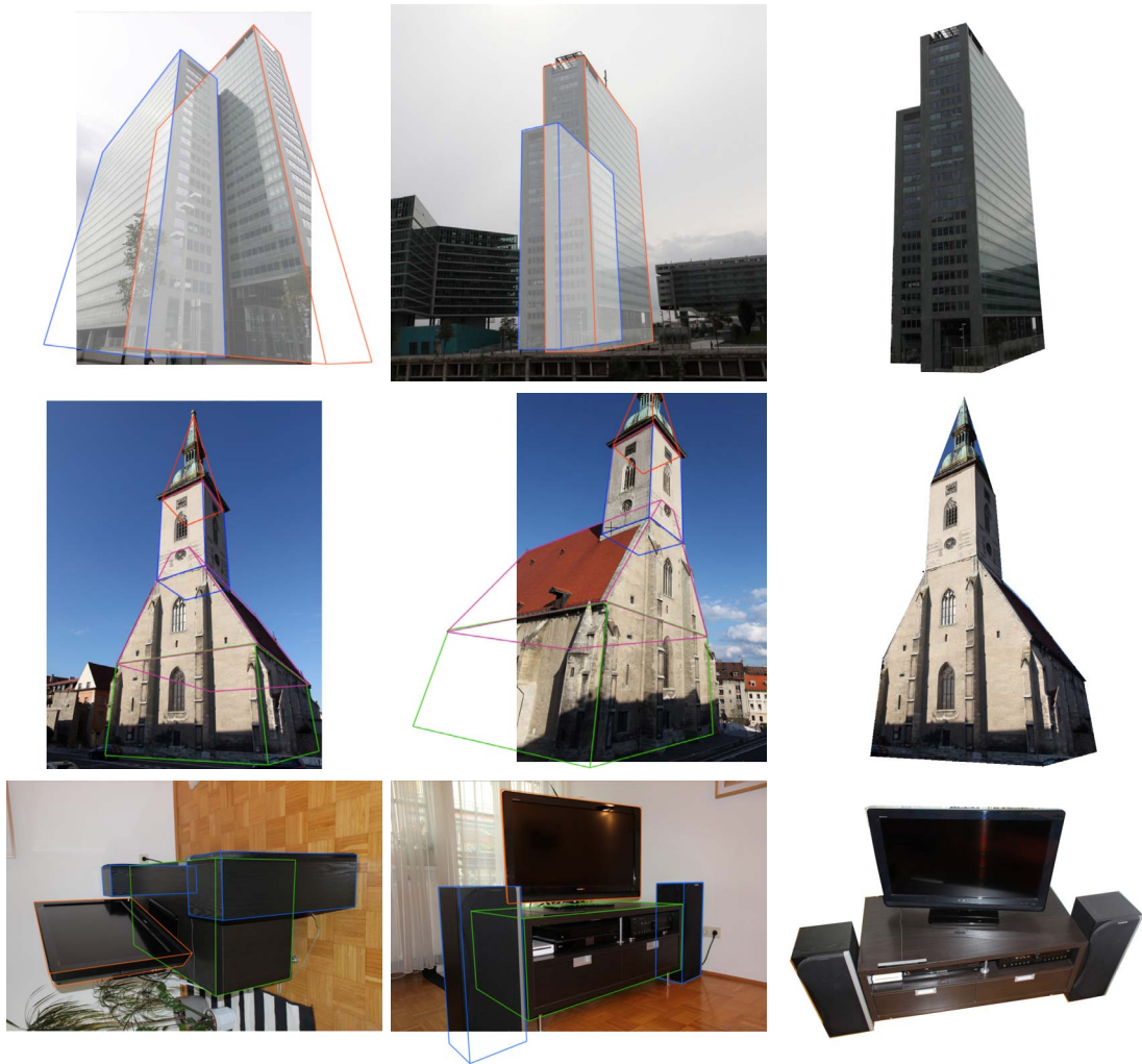
Figure 3.9: Top row: Edges in two images were used for generating the building model containing two boxes. Middle row: The church has been reconstructed with boxes, a frustum and a pyramid. The shape of the roof is too complicated for our model fitting approach, but it is possible to provide a simple approximation. Bottom row: The TV-set has been reconstructed from three images with three boxes and one frustum.
