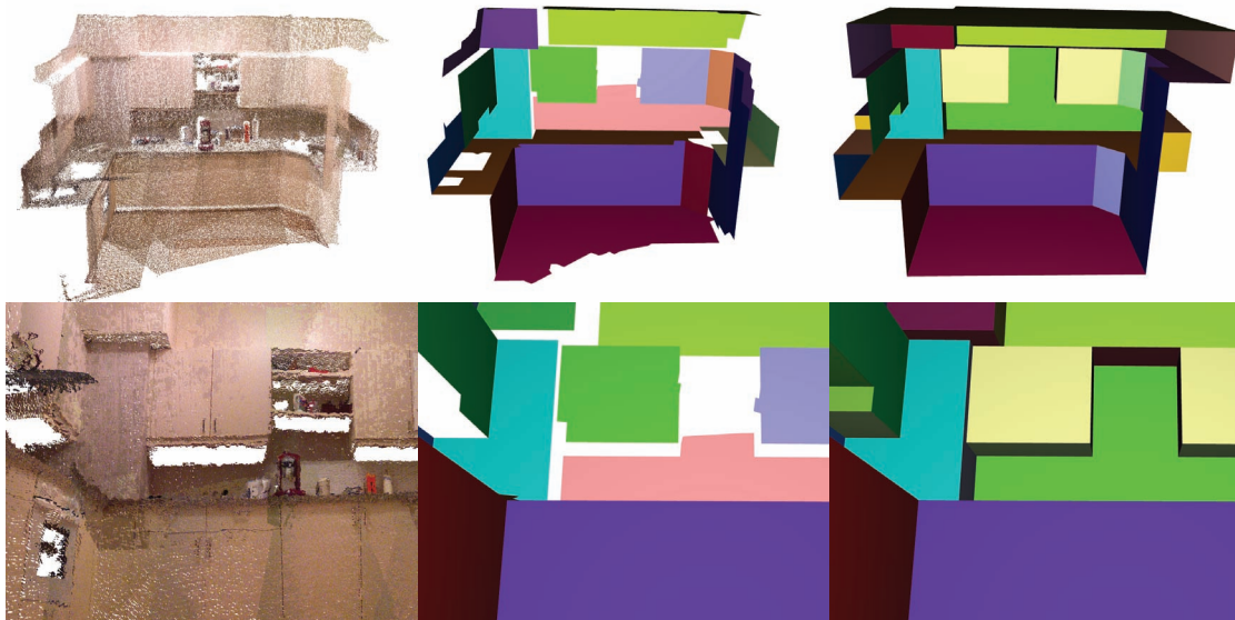
Figure 5.22: A point cloud from thirteen range images has been reconstructed with 26 shapes. Both rows show the input point cloud, the automatically reconstructed and the final model after some user inputs from different viewpoints.
