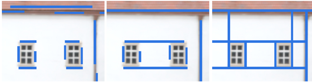
Figure 4.5: Nearly collinear line segments are merged (center image) and subsequently connected to form a grid (right image). Each line segment is elongated up to its nearest intersecting line.
