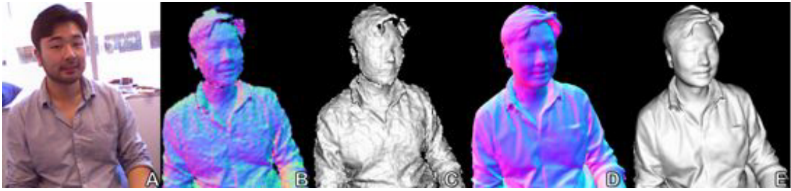
Figure 2.6: KinectFusion: A) RGB image. B and C) Normals and 3D Mesh from single depth map. D and E) 3D model generated from fused TSDF [61]. ©ACM.
