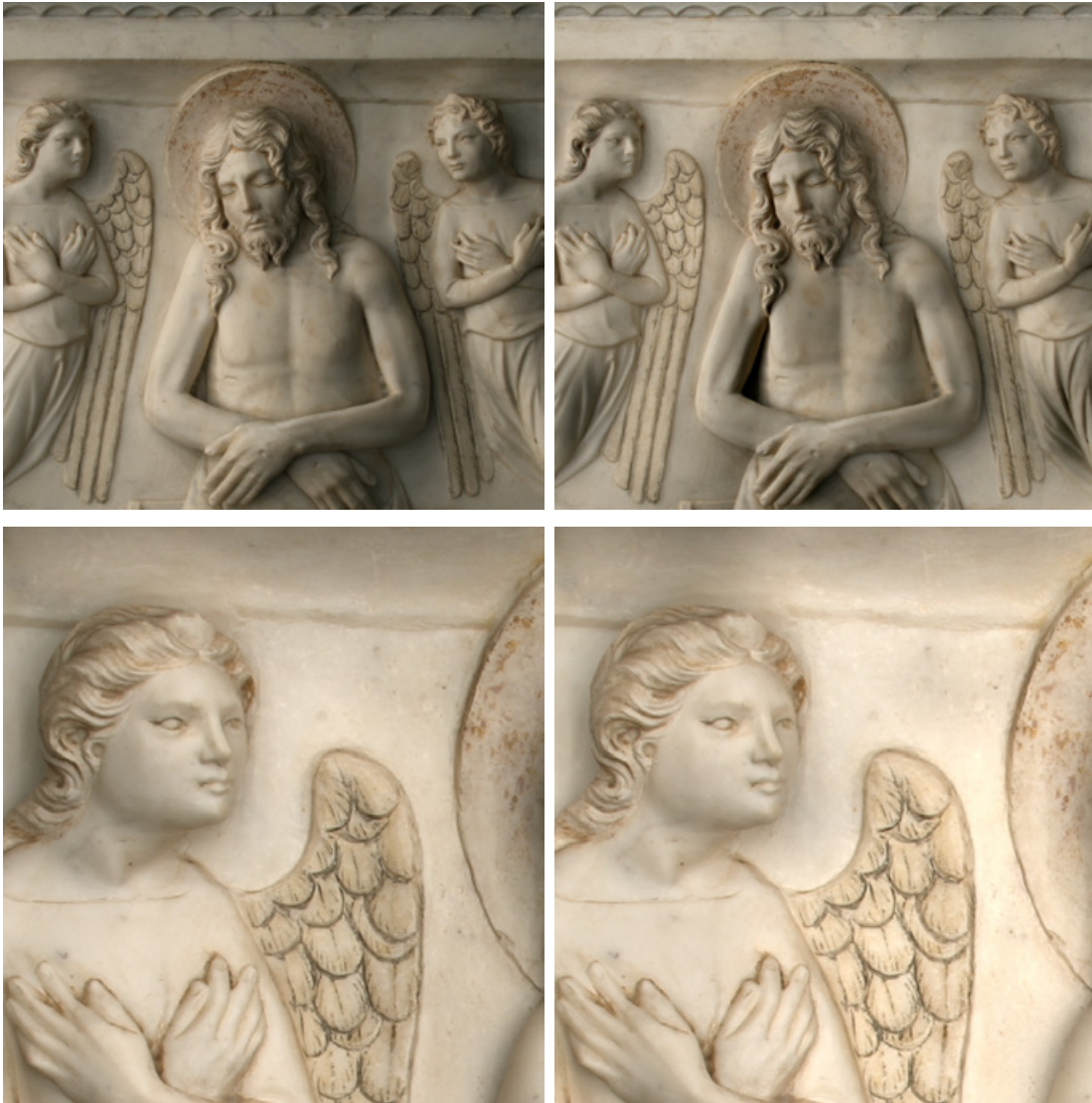
Figure 6.7: Dynamic Multi-Lighting Enhancement with anisotropic sampling. (Left) Standard rendering. (Right) Dynamic Detail Enhancement with (\alpha = 0.7) . Changes in scale are automatically achieved thanks to the view-dependent nature of the algorithm.
