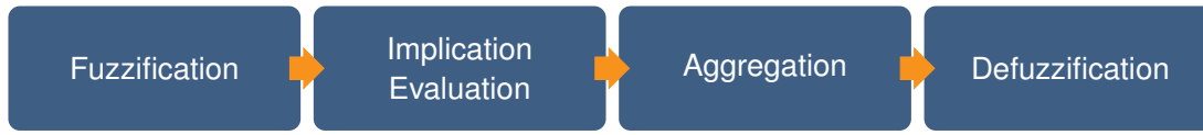
Figure 4.5: Common workflow of a FIS. First, crisp input values are fuzzified using fuzzy membership functions. Second, the antecedents of the if-then rules are evaluated using fuzzy set operators. The implications are evaluated with the minimum operator [97]. Third, the fuzzy implication results are aggregated and, fourth and finally, defuzzified using the centroid method to provide a crisp output.
