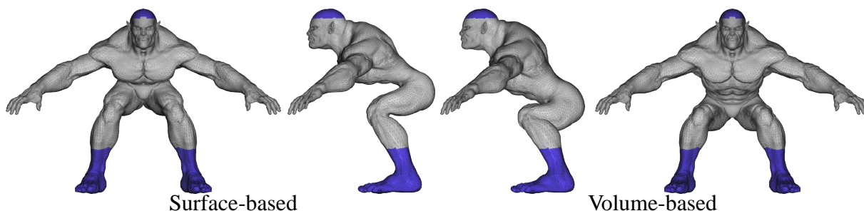
Figure 8.19: Self-intersections in the otherwise clean Beast prevent volume-meshing with previous methods. Surface-based deformation is one option, but bending causes shell-like collapses not present in a volume deformation enabled by our method.
