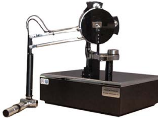
Figure 1.3: A 6 degree of freedom (DoF) haptic device, the Sensable Phantom Premium.
