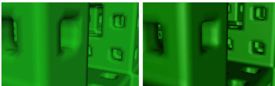
Figure 3.15: A close up view of a Menger Sponge dataset. The image to the left shows the render using an extracted isosurface with nearly eleven million triangles. The image of the right shows the direct volumetric isosurface rendering of the same dataset.
