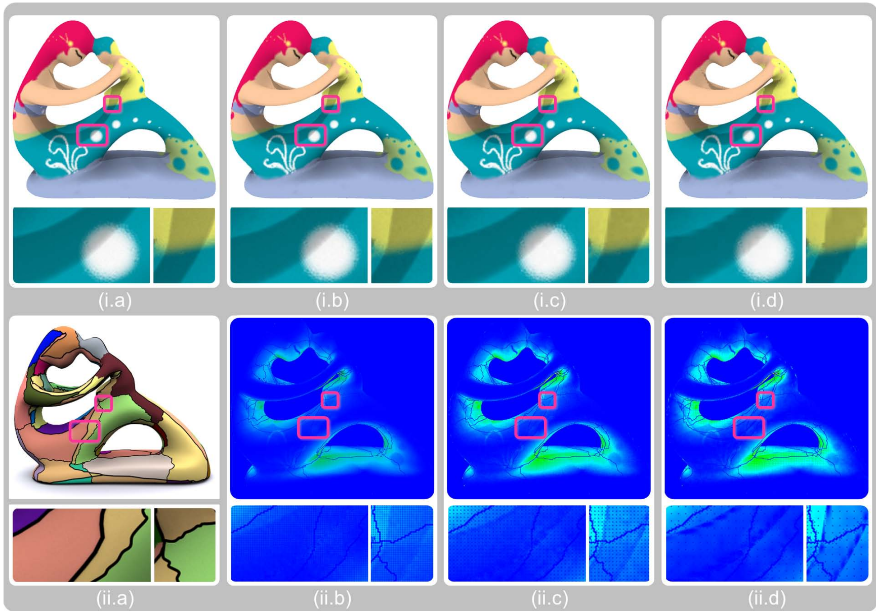
Figure 78: Quality depending on the number of passes. Top row: Ray Tracing reference and 2, 3 and 4 passes respectively. Bottom row: the clusters and the respective error images. The insets show details of the texturing and soft shadows.
