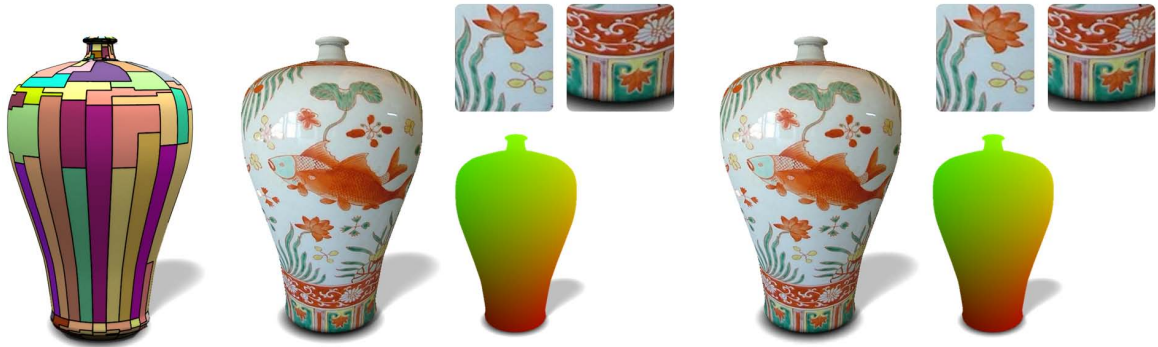
Figure 81: Correct texture rendering. Left: clusters, Middle: Ray Tracing, Right: I-render. The lower insets show the smooth interpolation of the texture coordinates.
