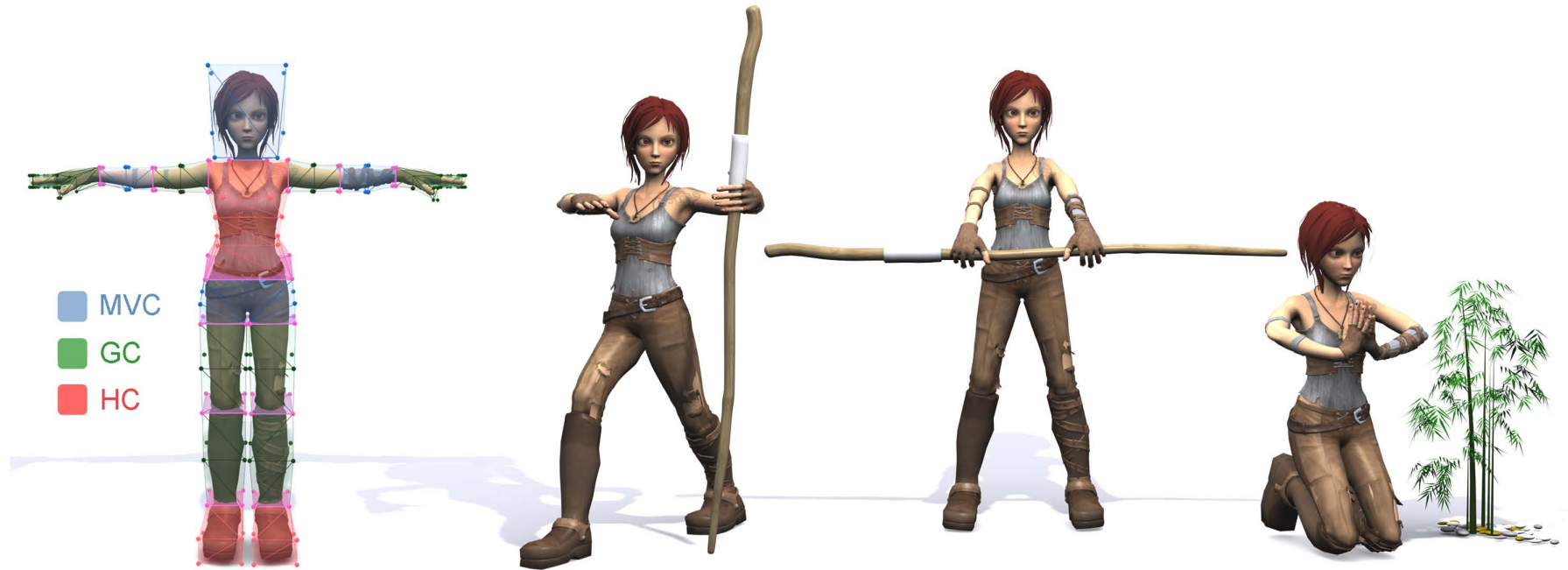
Figure 67: Deformations of the Sintel model (66845 triangles) using *Cages. Left: Cages at binding time with different coordinates (Blue - MVC, Green - GC, Red - HC, and pink cage boundaries). Right: Composition of different poses.
