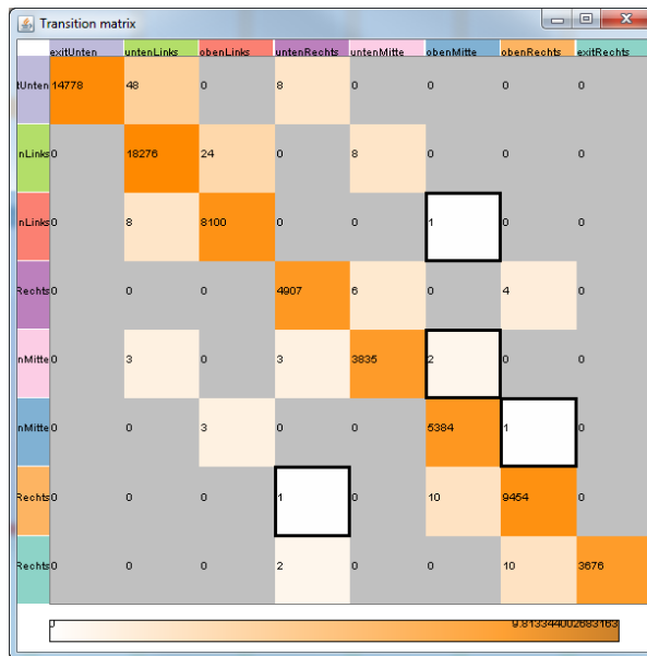
Figure 9.4.: The transition matrix is used to highlight the selected group changes. Thereby, rare transition can be identified and analyzed in more detail. In the matrix selected transitions are highlighted by a block border.
