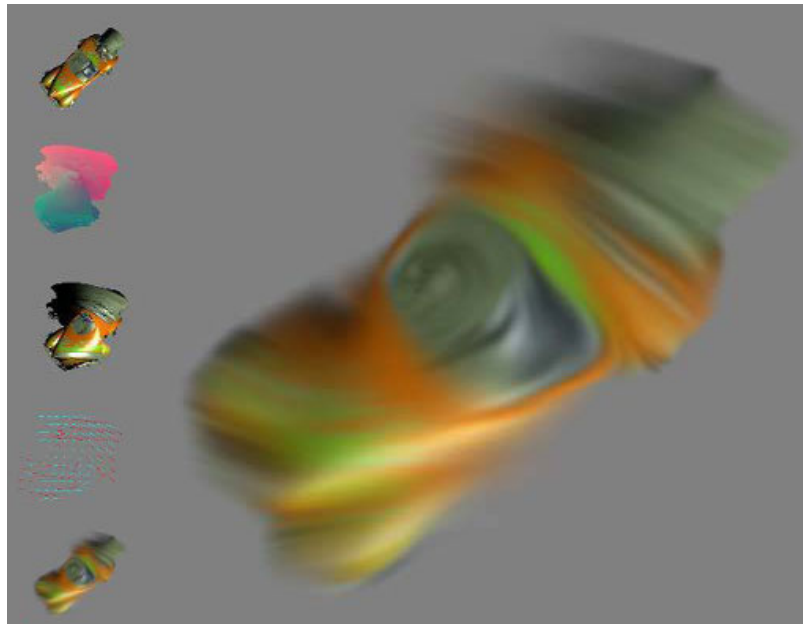
Figure 4.18: Real time motion blurred car using the method of Shimizu et al. [224]. Insets show, from top to bottom, a render of the original geometry, motion vectors, warped geometry, optic flow vector field and final rendered geometry.
