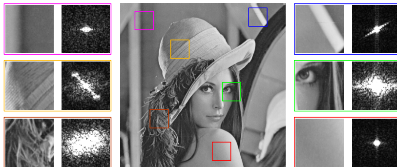
Figure 1.4 – The Fourier transform of a signal depicts its variations. We illustrate this notion using the Lena image. We select portions of the image and display the Fourier transform in insets. Low frequency regions of the image are compacted around the origin of the Fourier domain while high frequency regions distribute in the Fourier domain.
