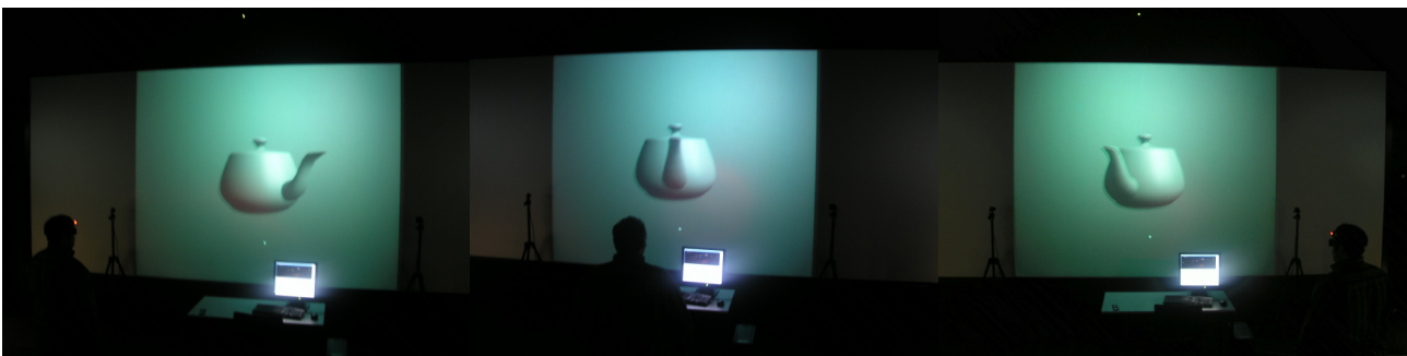
Figure 5.24: View-dependent visualization via robust head tracking, based on this algorithm. [Arn07]
