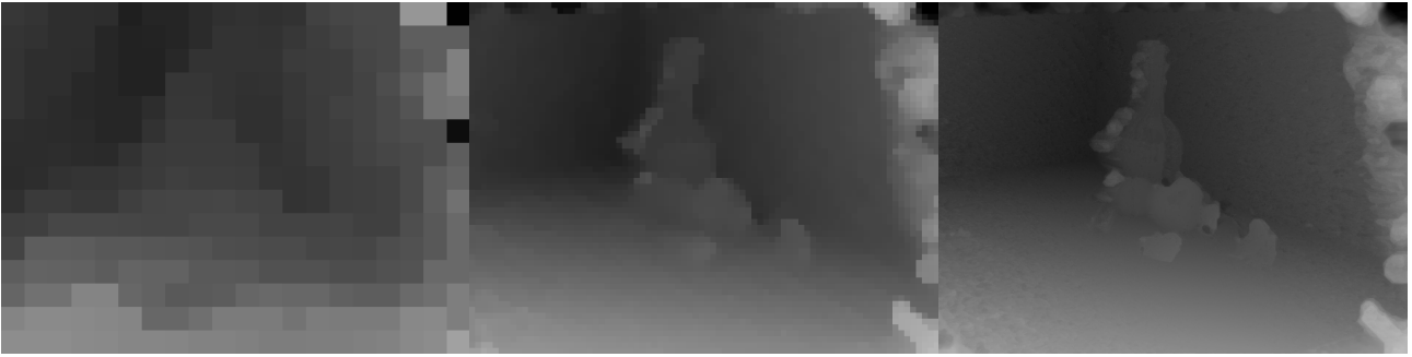
Figure 5.16: The importance of median filtering in depth hypothesis refinement.
