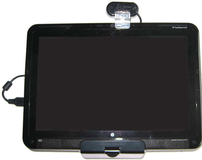
Figure 7.2.: The tablet PC is equipped with an additional webcam to act as see-through device.
