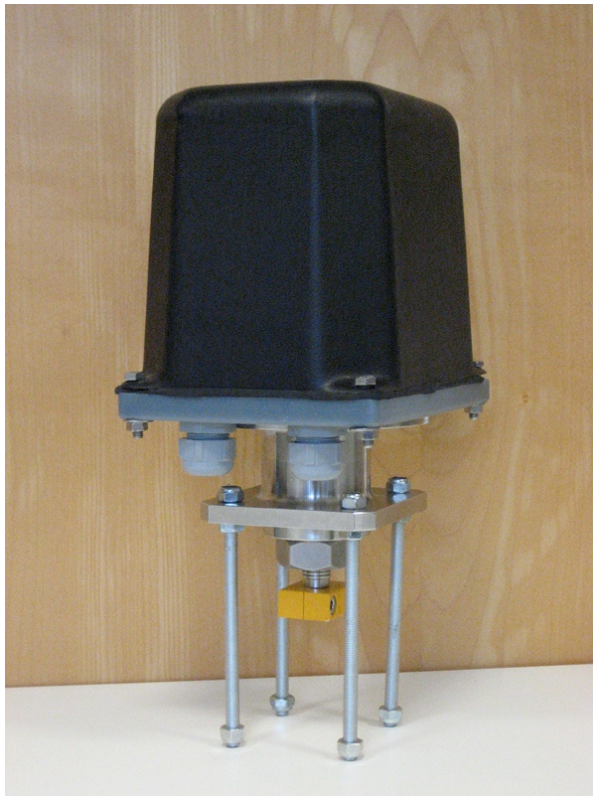
Figure 6.3.: The selected exemplary training scenario consist of replacing two sensors and the belt roller of this actuator. For this purpose the actuator must be partly disassembled and reassembled after replacing the damaged components.
