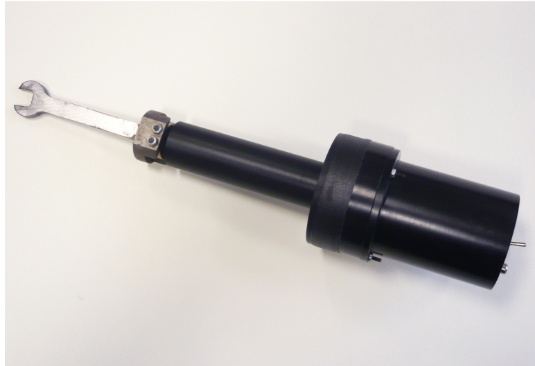
Figure 4.7.: Force-torque sensor developed by PERCRO (see also [TFR*10]).
