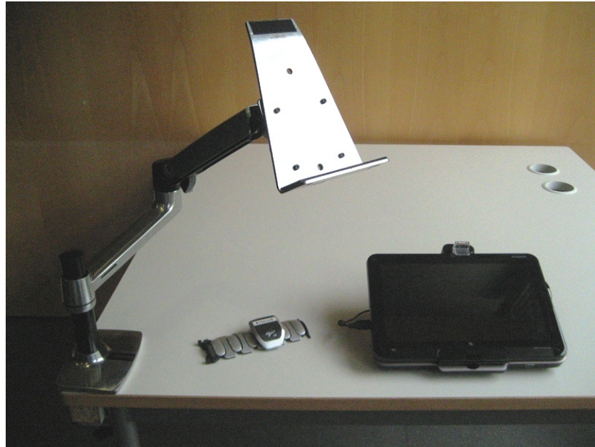
Figure 7.1.: Setup of the training platform: tablet PC equipped with a webcam, movable mount, and haptic bracelet.
