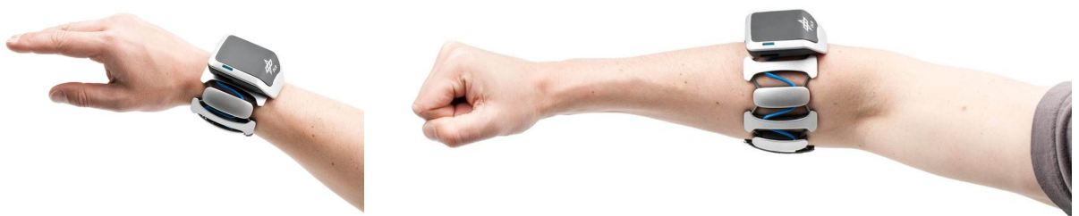
Figure 6.1.: A vibrotactile bracelet developed by DLR (German Aerospace Center) [SEWP10].
