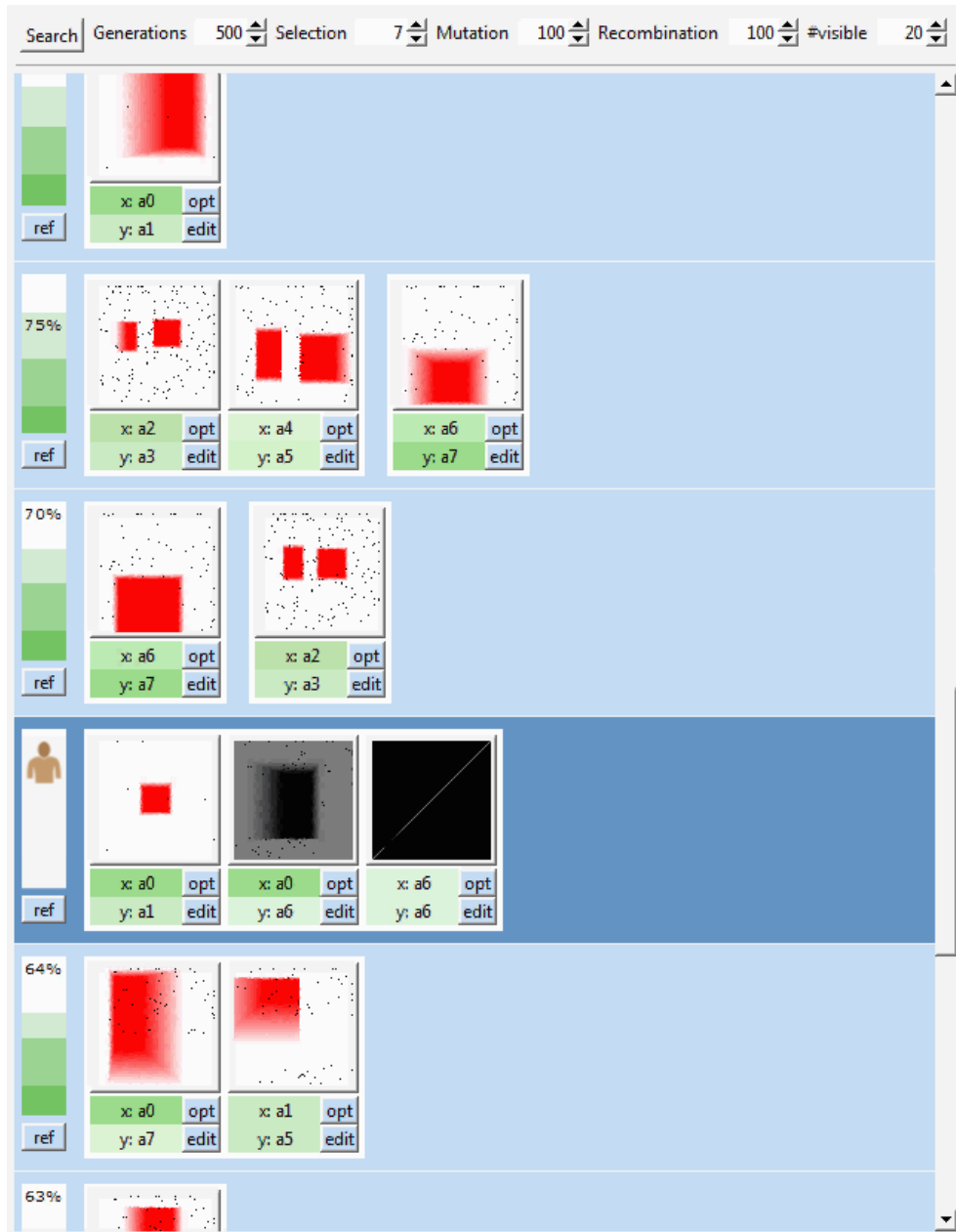
Figure 5.1 – Interactive visualization of hypotheses that have been found by a genetic search algorithm. A hypothesis is a combination of fuzzy-logic selections to explain features in the simulation data.
