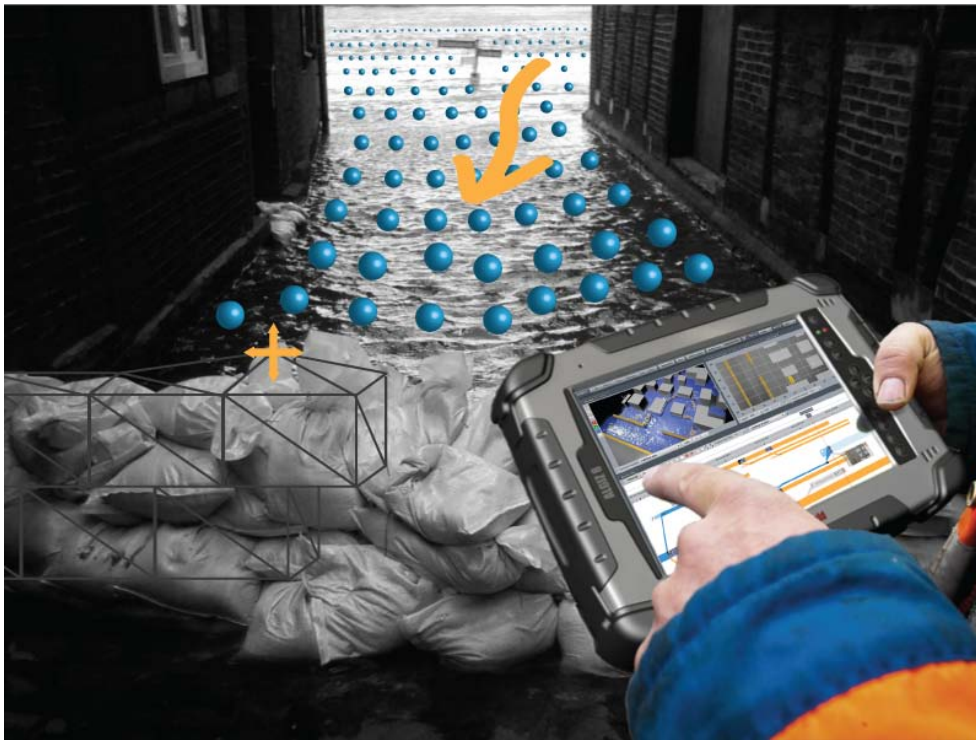
Figure 1.5 – Future application that envisions the presented system in an online mode during a flood event (mock-up). A first responder on-site consults the mobile client of the Visdom application for designing a temporary flood protection. The remote server is in charge of evaluating the compute-intensive parts of simulation and visualization.
