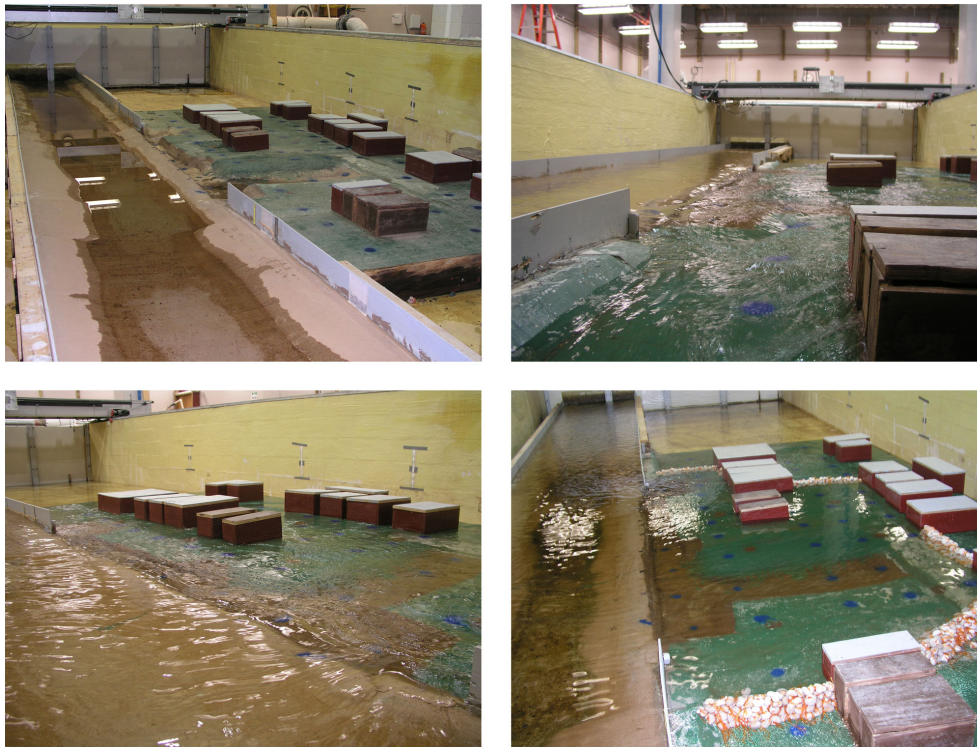
Figure 1.3 – Recreation of the levee-breach scenario in a hydraulic laboratory. Researchers study alternative barrier arrangements to accomplish a successful breach closure [112].
