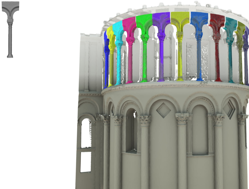
Figure 5.11: One column has been extracted from the apse of the Pisa Cathedral (upper left). In combination with an isometric mapping with six degrees of freedom (translation and rotation) it forms a “degenerative” model. The fitting algorithm minimizes the objective function, which defines a measure of similarity; i.e. it identifies “copies” of the reference. Each “copy” is rendered in a different color and blended with the input data set.
