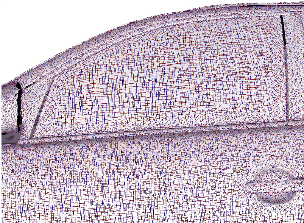
Figure 4.52: Going by curvature flow simplifies the patch layout for a human modeler. In this way the modeling task can be performed more efficiently.
