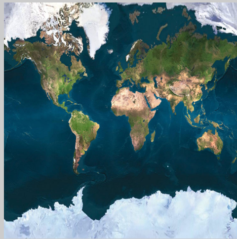
Figure 3.14: The MERCATOR map is an angle preserving map; i.e. angles measured in real world and measured in the map are equal. This is an important property for navigation.
