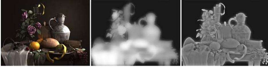
Figure 4.1: Left: Input image (synthetic render of a still life (LMJH + 11)). Middle: Base layer. Right: Detail layer.
