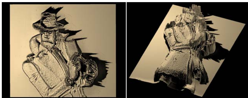
Figure 8.3: Recovered depth from a given image. Errors remain mostly unnoticed from the original viewpoint (left), but become more obvious if it changes (right). Light and shadows have been added for visualization purposes.
