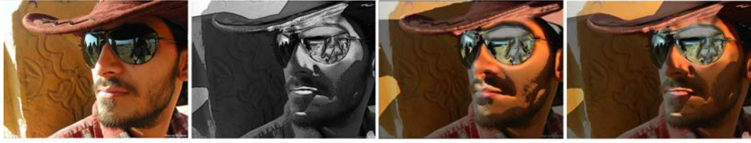
Figure 8.13: Example of depth editing. From left to right: Input image and relighting result with light source at (550,400,460) , image obtained with automatic depth map generation and after being edited by an artist with our tools for 5-10 minutes. The retouching tools helped in both correcting noticeable mistakes from depth generation (the emboss effect of the sunglasses) and creating a more interesting combination of shading and shadows (nose, lips, cheeks, jaw, ...).
