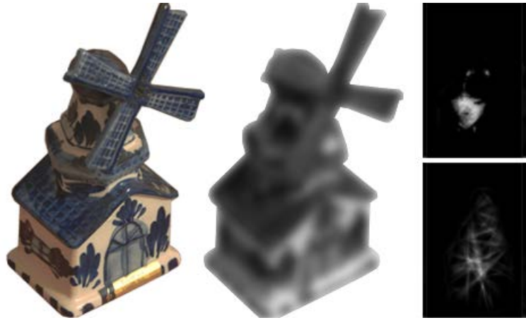
Figure 7.4: From left to right: segmented mill from Figure 7.1, recovered depth map (KRFB06) and two maps with 1 and 20 orientations respectively.
