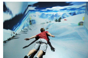
Figure 6.71: PPRacer, an open source game ported to the DAVE with the Davelib. The penguin is controlled by the user's head position.
