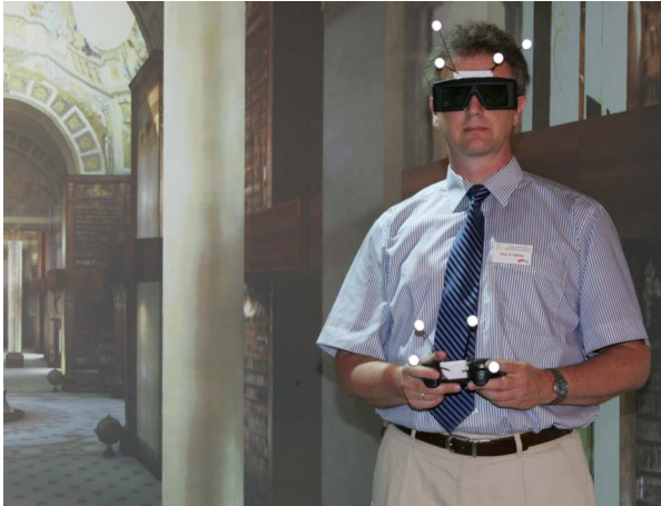
Figure 2.52: Tracked gamepad and 3D glasses as input devices in the DAVE in Graz.
