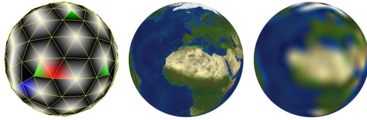
Figure 6.33: Icosahedron subdivision for spherical wavelets on a sphere. Visual debugging and testing of finding neighbor vertices (left), loading an image texture (middle) and applying a blur by setting wavelet coefficients of a higher level to zero (right).
