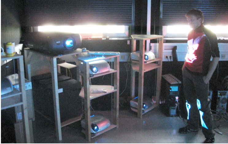
Figure 2.34: Most of the HEyeWall projectors: 6 small tiles and one large projector covering the whole screen.
