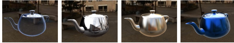
Figure 6.62: A few shader materials that also work correctly in the DAVE with stereo and head tracking. As an example, a mirror reacts on head motion and shows correct depth. To include head tracking, the shaders and their setup need to be adapted. Reflections are only approximated with an environment map computed for one point of view. A second diffuse version of this map can be used to obtain a diffuse reflection without a loss of performance.
