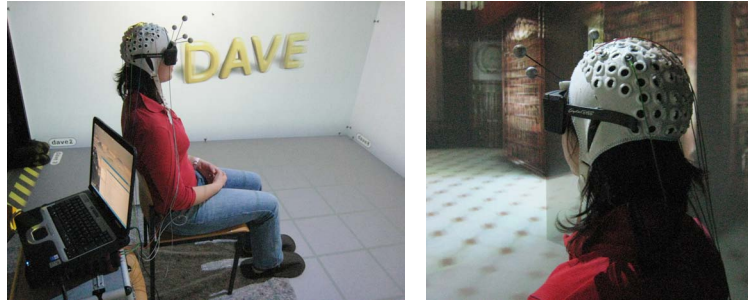
Figure 2.32: The brain computer interface (BCI) and a test subject in the DAVE. Electrodes are placed on the head to measure electroencephalogram (EEG) signals. Recognizing previously learned patterns, the subject is able to navigate through a 3D scene in a very limited way.
