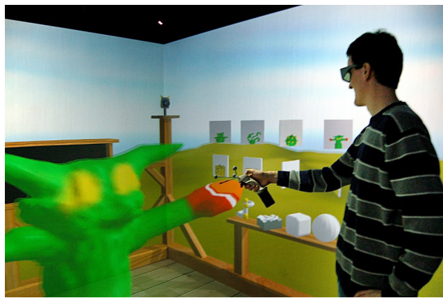
Figure 6.54: Triangle mesh modeling tools for the DAVE. Left: The result of a 2.5D terrain. Left: Sculpting is performed by surface extrusion and dynamic retessellation. On the right side, a set of tools can be selected or previously saved models can be loaded.
