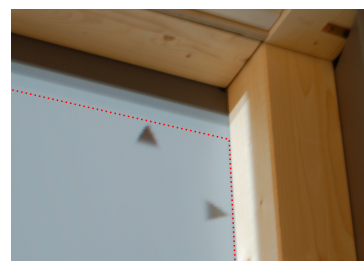
Figure 4.6: The projection slightly overlaps the screen area visible from the inside of the DAVE, indicated by a red dotted line. The current calibration is also visualized by the system background image, that is recomputed accordingly after each calibration.
