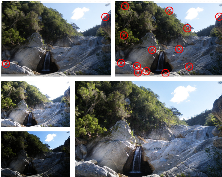
Figure 6.14: Photo Distorter. Top row: Rotation, translation and scale are adjusted, defined by two control points. Some ghosting remains (left) vs. free-form deformation with more control points (right). The two small images on the bottom left are the original input images, the bottom right shows the final tone mapped result using the free-form alignment.
