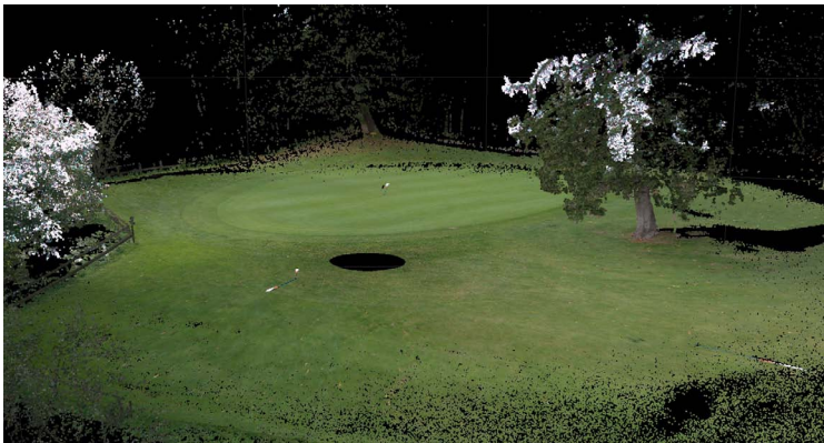
Figure 6.65: Point cloud viewer, showing a LIDAR scanned scene of a golf court near Graz. The original full resolution scan contains 50 million points, only 10% random samples are used here for visualization. The scanner was placed on a tripod near the center of the image (black hole). Close to the scan location, the point density is very high. Scan shadows are visible e.g. at the right side, where geometry was occluded by the tree. To obtain a color, photos can be registered to the scan. The bright areas in the trees show sky color due to a misregistration.
