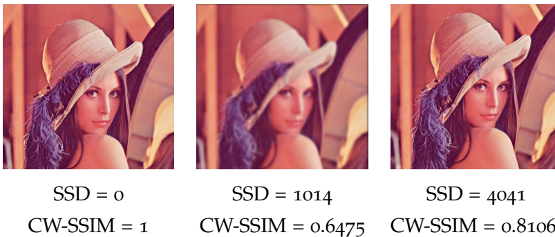
Figure 54.: The human visual system is more susceptible to local errors than to global ones. Even though the right image, which is a shifted version of the original on the left, has a four times higher sum of squared differences error (SSD) than the blurred one in the middle, we would prefer the shifted version. This is also confirmed by the complex wavelet structural similarity index (CW-SSIM) [257], which gives a better approximation of perceptual image quality. All values have been computed on the luminance channel.
