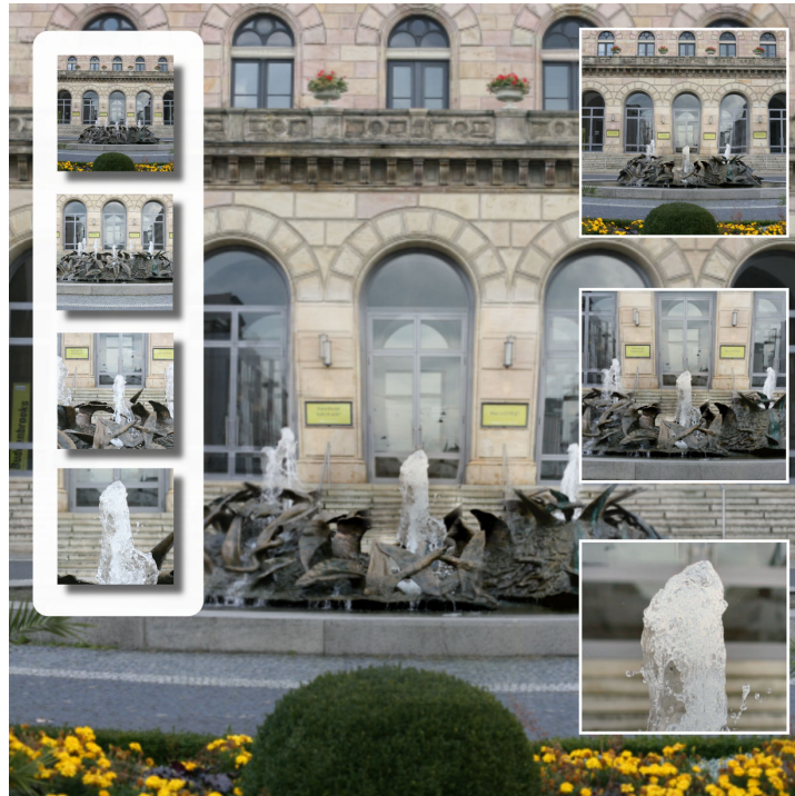
Figure 35.: Zipmap of a facade with fountain. Time-varying parts of the scene are merged into a common representation. Four input images of size 512 \times 512 pixels are used to create a virtual resolution of 20 megapixels in the central portion of the scene.
