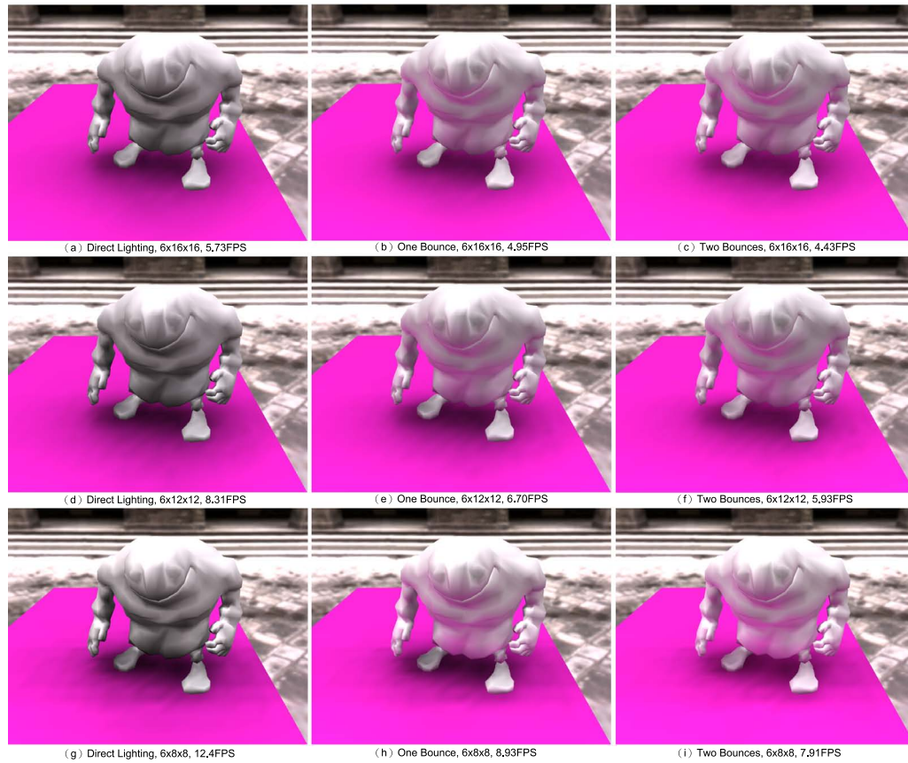
Figure 4.8: A monster rendered under environmental lighting with direct illumination, one-bounce, and two-bounce indirect illumination and varying discretizations (3378 vertices).
