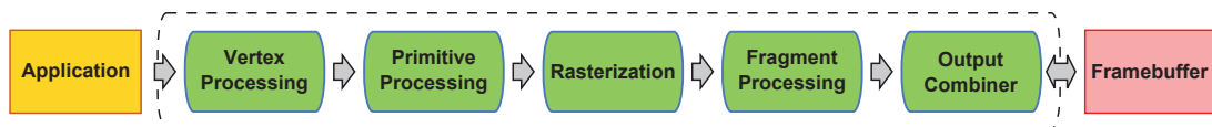
Figure 2.1: The Graphics Pipeline. The rendering process is started by the application , which sets up and issues the drawing command, sending to the graphics system data such as vertex attributes, connectivity information, material properties and viewing parameters. Data flows through the whole graphics pipeline to the framebuffer , a memory region that holds the final raster image.
