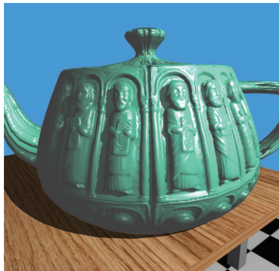
Figure 2.25: Relief Mapping: Arbitrary Surfaces. By working in the polygon tangent space, relief mapping can be applied to arbitrary polygonal meshes.
