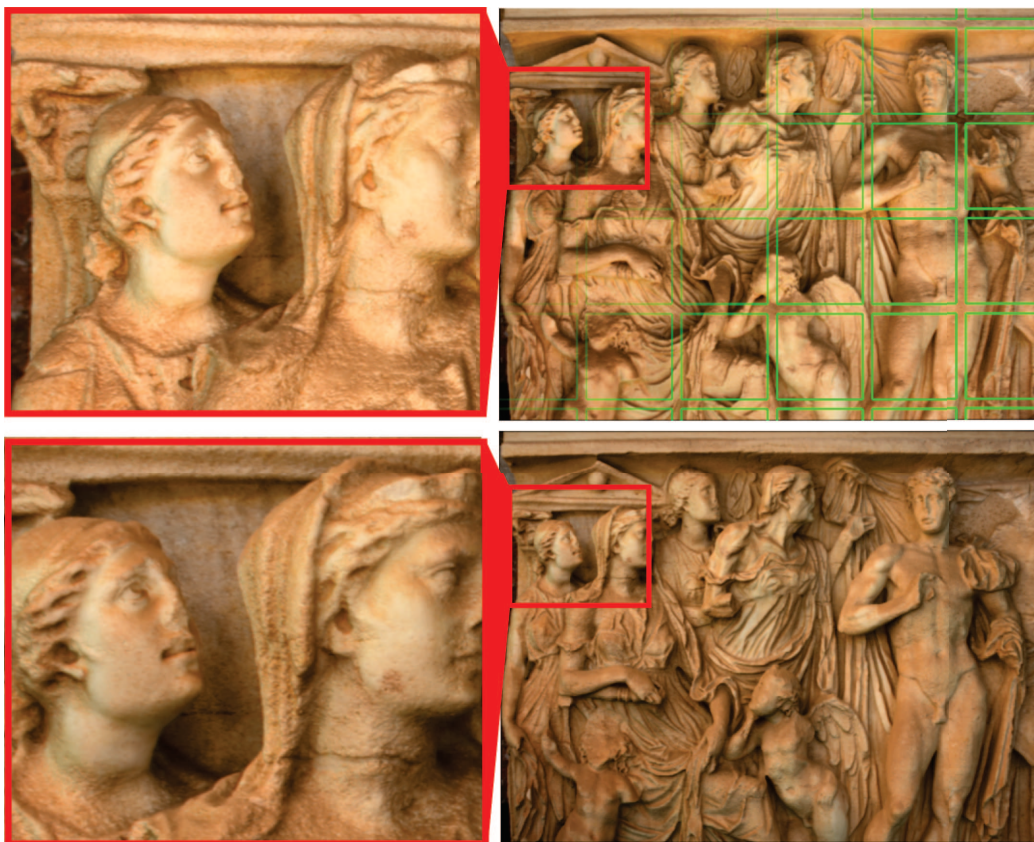
Figure 5.8: Polynomial Texture Maps. Four frames captured when visualizing a High Quality PTM. Light position is bound to the position of the mouse on the window.
