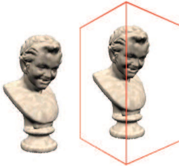
Figure 2.22: Rendering with Relief Mapping. A view-independent impostor of a statue is rendered by only drawing the object bounding box with pre-warped relief maps.
