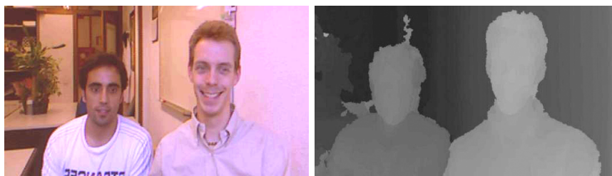
Figure 2.13: Depth image (right) for a given scene (left).
