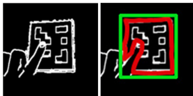
(b) Edge segmentation (left) and Candidate Detection (right).
