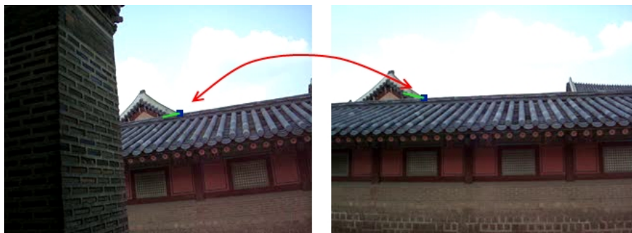
Figure 3.7: A false corner indetectable by the Kalman Filter
