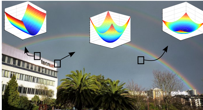
Figure 3.3: Different responses of the Harris detector 1 .
