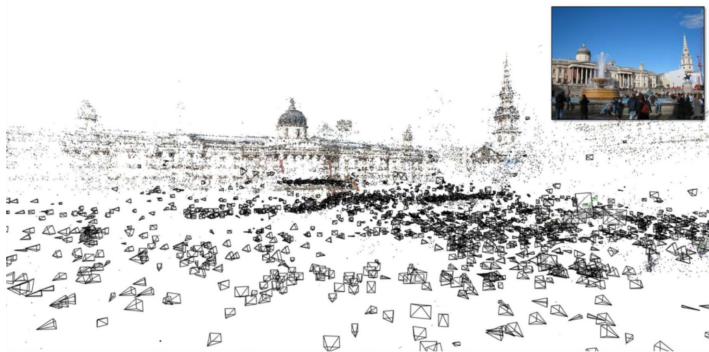
Figure 2.6.: Comparison of a photo to a sparse reconstruction of a huge number of unordered photographs. Figure courtesy of [SSG*10].
