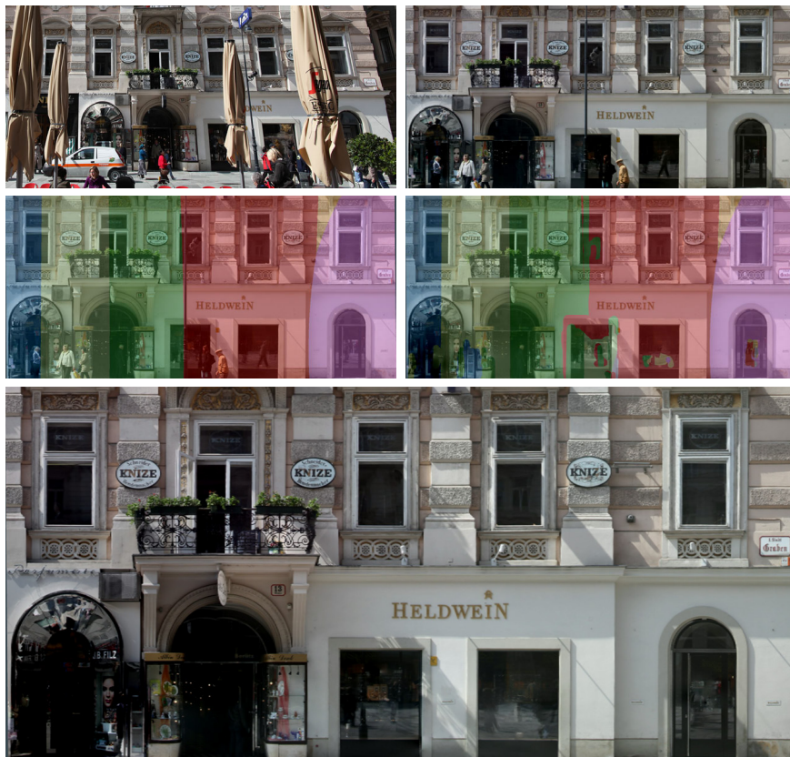
Figure 3.10.: Steps of the multi-view image generation system. Top-left: one of typical perspective input photographs, please note the occlusion. Top-right: the result of the proposed ortho-image generation method (note the pedestrians). The second row shows masks indicating source images of the composition by colors: automatic result (left) and interactively post-processed (right). Bottom: the final result after interactive post-processing.
