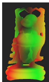
Figure 5.3: The frame-to-frame optical flow using color coding for a rotating Happy Buddha. The fixpoint of the rotation is visible as a dark spot.
