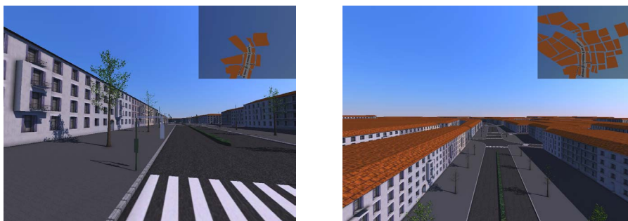
Figure 1.2: (left) Using visibility culling, we send only the visible buildings bordering to the street (shown as red roofs in the small overview window) to the graphics card for a low view point. (right) This is only a fraction of the buildings rendered for a high view point.
