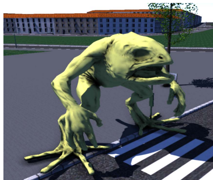
Figure 6.1: As can be seen in this snapshot, our real-time-rendering framework features techniques like shadow mapping and SSAO for realistic lighting (i.e., quantitative visibility). The core rendering algorithm uses visibility culling for acceleration (i.e., qualitative visibility).
