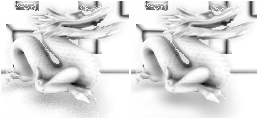
Figure 5.10: Rotational movement using TSSAO. (left) Without filter. (right) Using our filter. Note how the filter is only applied in the noisy regions, while the rest stays crisp (Zoom into the pdf to see the differences).
