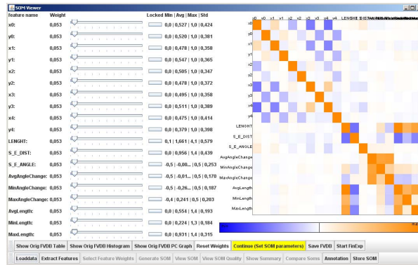
Figure 4.26.: Interactive selection and weighting of trajectory features determining the similarity calculation. From left to right in the picture: Feature names, current feature weights, weight adjustment interface, basic feature statistics, feature correlation matrix with color scheme from blue (-1) to orange (1).
