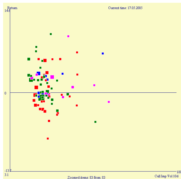
Figure 4.12.: Visualization of the time data in a scatterplot showing a snapshot of the data in a single time point. The x-axis and y-axis encode the two dimensions of the data. Additional dimensions, if provided, are displayed using color and glyph size. Animation is used to represent the time-dimension of the data.
