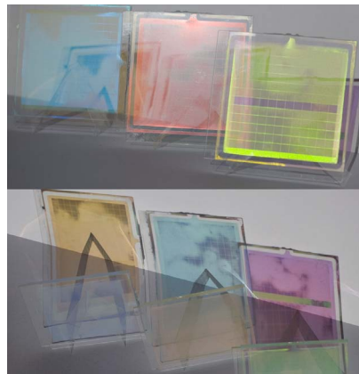
Figure 5.6: Three lab samples of bistable cholesteric liquid crystal panels in reflection (top) and transmission (bottom). The green panel has one row of pixels set to transparent. Similar technologies could be used for additional colour modulation in a multi-layer BRDF display.
