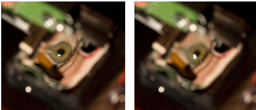
Figure 5.17: Reflection of a human eye in Setup 2b filled with liquid metal. Left: resting. Right: in motion. The distortions are caused by surface tension.
