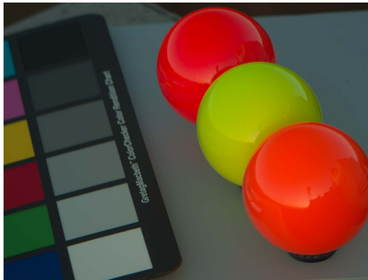
Figure 4.3: Spheres covered in three different multilayer paint varieties for utility vehicles (“pearl white” primer, fluorescent red/yellow/orange paint, clear coat). Note the outstanding chroma of the paints, and their luminance, which even in the non-specular part is higher than the one of the 90% white ColorChecker patch.
