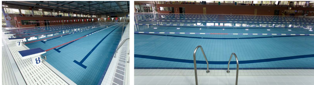
Figure 3.10: Two views of an olympic swimming pool. Note how the nonlinearity in Snell's law introduces severe geometric distortions. On the left photo, the refraction causes apparent intersections of lines that are in fact parallel.
