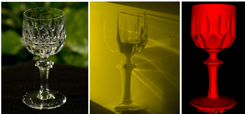
Figure 3.1: From left to right: Photo of a glass goblet, light sheet in fluorescent immersion intersecting the object, reconstruction from 6 scans under different orientations.
