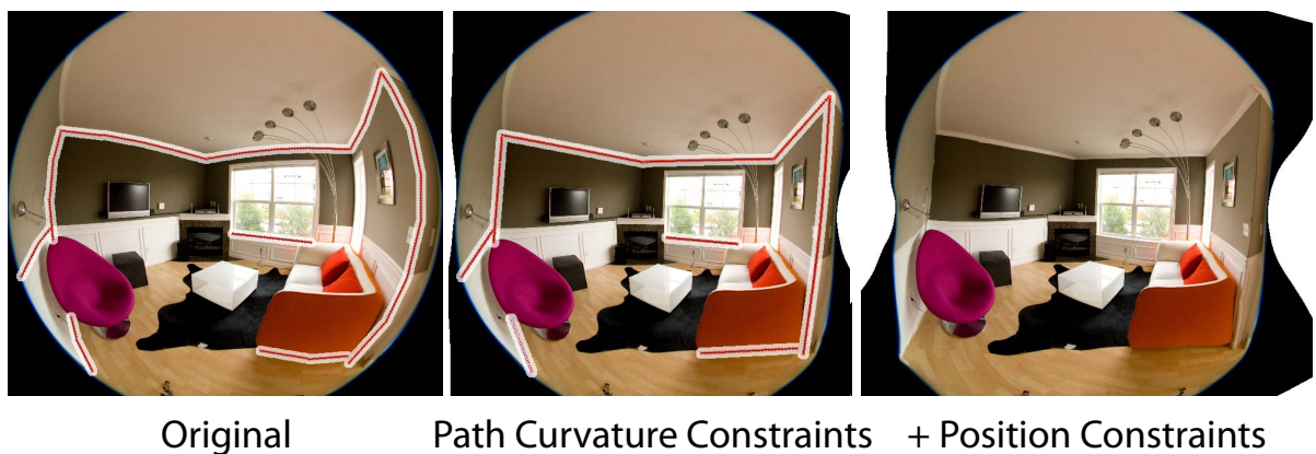
Figure 3.15 Correct "fisheye" lens distortion by combining path curvature and position constraints. (Original image taken from [CAA09] and kindly provided by Aseem Agarwala.)
