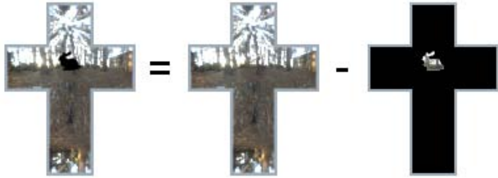
Figure 5: The irradiance I_p arriving at a point p that lies under the bunny (left), is equal to the total irradiance I_{tot,p} (middle) minus the irradiance intercepted by the bunny I_{occ,p} (right).
