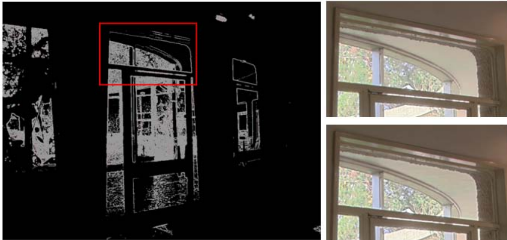
Figure 37: Depending on the level of importance_{threshold} used, the selective tonemapping (top-right) may under-performs comparing to the ground truth local tonemapping output. Important areas map with superimposed VDP map (red dots) is given on the left.
