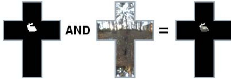
Figure 8: The binary mask denoting the part of the environment map covered by the occluder (left) is ANDed with the environment map (middle) to get the occluded part of the environment map (right).
