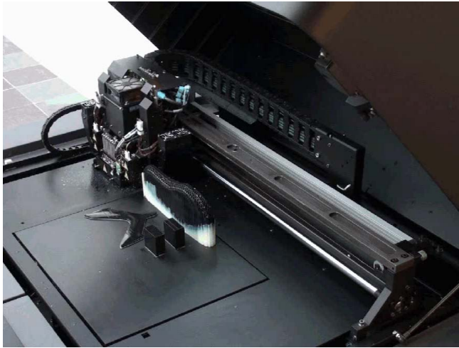
Figure 8.7: Objet Connex 500 3D multi-material printer. Image: Final result after approximately 10 hours printing. White material is support material which is removed using a high-pressure water jet. Table: Build resolution of the printer in high-quality mode [OBJET, 2009].
