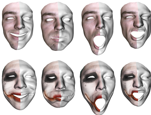
Figure 1.5: Accurate 3D facial expressions can be transferred in real-time from an actor (top) to a different face (bottom).
