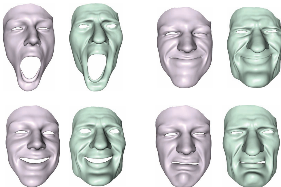
Figure 5.14: Bringing an ancient Roman statue to live. The actor (magenta) can control the face of Caesar (green) that has been extracted from a laser scan of the statue.
