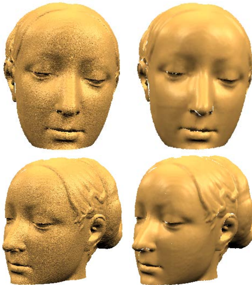
Figure 3.7: Smoothing of two range scans of the Ippolita Sforza Bust. Note that details in hair, mouth and eye regions are accurately preserved.
