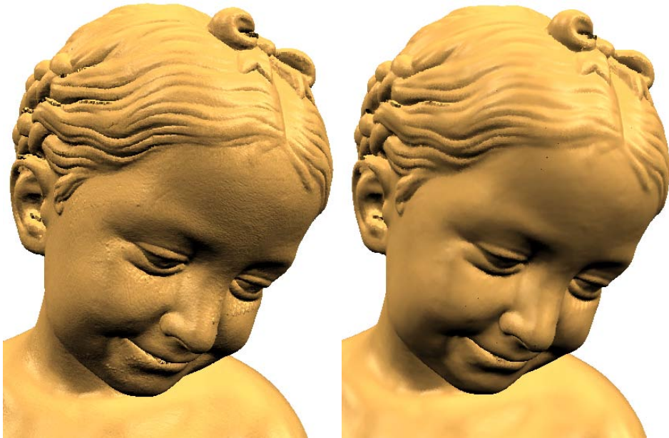
Figure 3.8: Left: Raw registered range data of the Bimba model obtained using a laser scanner. The data is corrupted by dense small-amplitude noise and scanning artifacts close to the mouth and the right eye of the model. Right: The artifacts are well dampened and noise is removed after filtering with our method.
