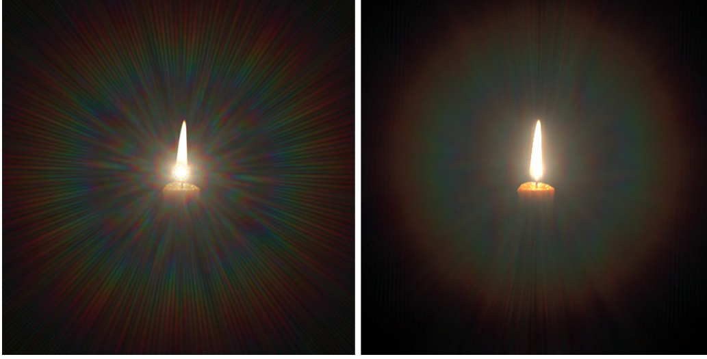
Figure 8.10: PSF applied using (left, 52.4 fps) billboards and (right, 30.2 fps) the convolution proposed. The results are substantially different for this candle. Using convolution, the horizontal needles of the ciliary corona blur out while the vertical needles remain unaffected.
