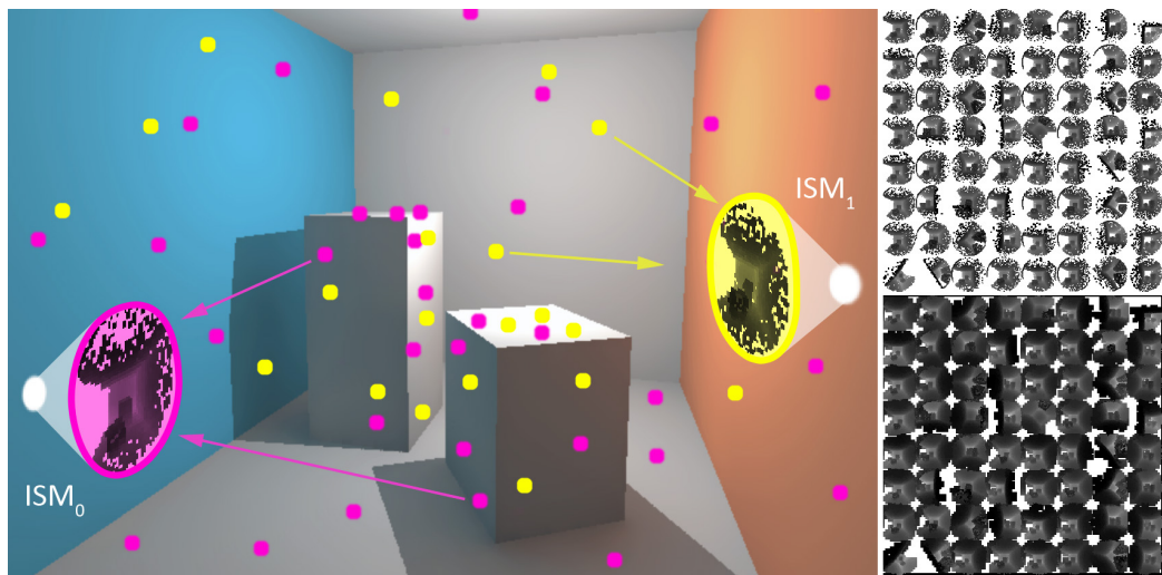
Figure 5.3: Global Illumination with imperfect shadow maps: The indirect light in this didactic scene is represented by two VPLs. Each VPL generates a shadow map using a point-based representation of the scene. Since coarse visibility information is sufficient, each VPL uses only a sparse subset of the points (encoded as colors) to generate an imperfect shadow map at real-time rates. The contribution of all VPLs is summed up yielding the final indirect illumination. Examples of imperfect shadow maps (bottom with and top without pull-push) are shown on the right; dark value signify small depth values and light values represent large depths.
