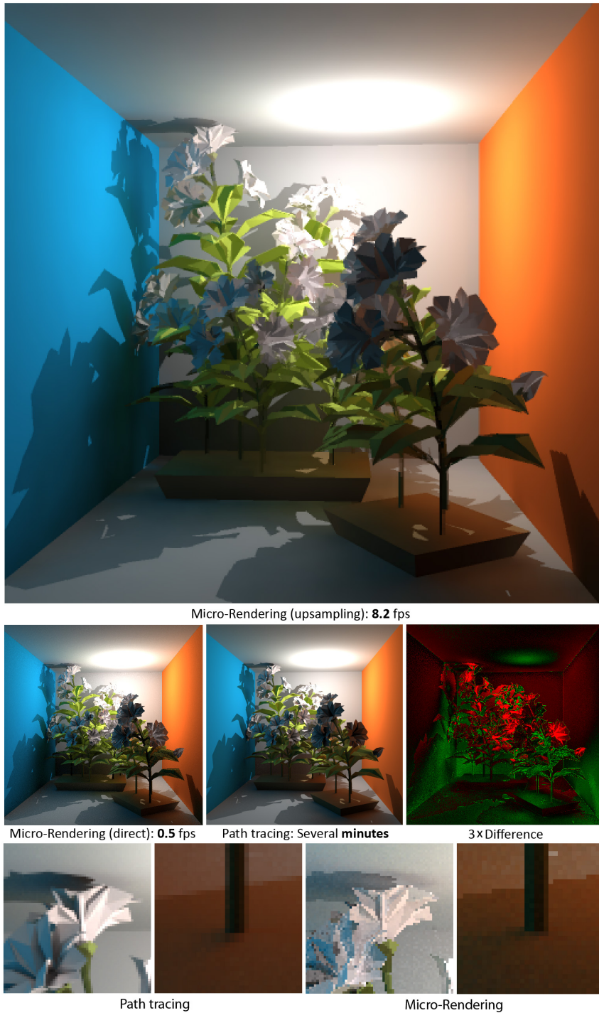
Figure 6.11: The geometrically complex plant scene shows some slight differences (see insets), which can be attributed to the discrete micro-buffers.
