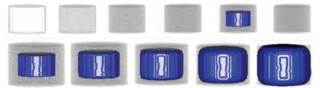
Figure 10: Top row shows volume rendering with cylinder cyl_8 classified. The bottom row shows the dilation steps for the cylinder.
