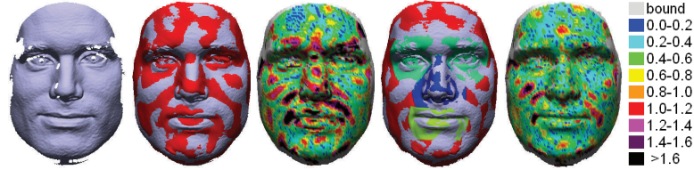
Figure 6.5: Redundancy estimation. From left to right, the face scan, S_{single} , the residual errors of S_{single} , S_{mult} , the residual errors of S_{mult} , and the color map for the point-to-point distances (in mm).
