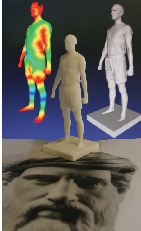
Figure 1.10: Colored geodesic measurements on the author’s reconstructed body surface effectively show the boundaries of the model. When the surface is made watertight, a 3D laser printer can turn the model into a real world object.
