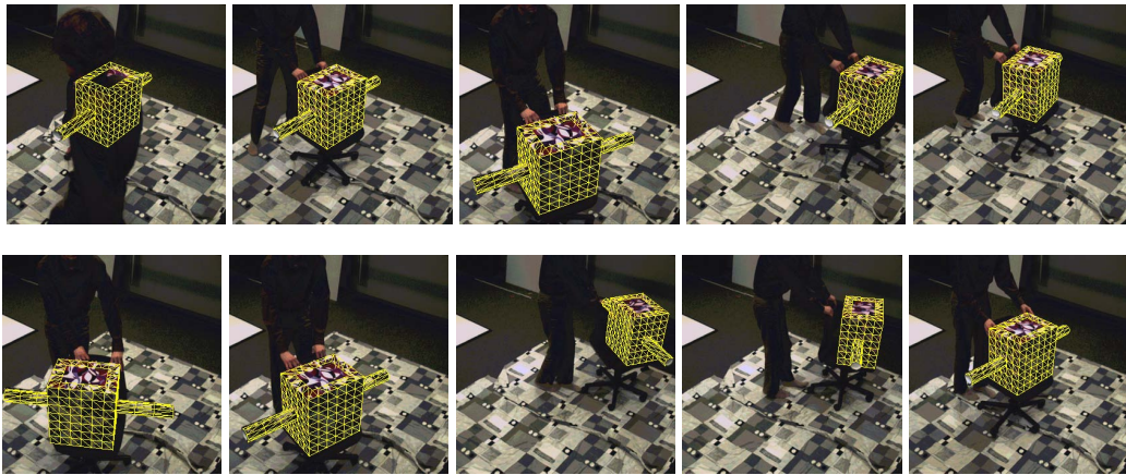
Figure 5.24: Pose estimates for 10 of 570 frames. The sequence contains several difficulties for tracking: a rich textured and non-static background, shadows, occlusions, and other moving objects. Only one camera view is shown.
