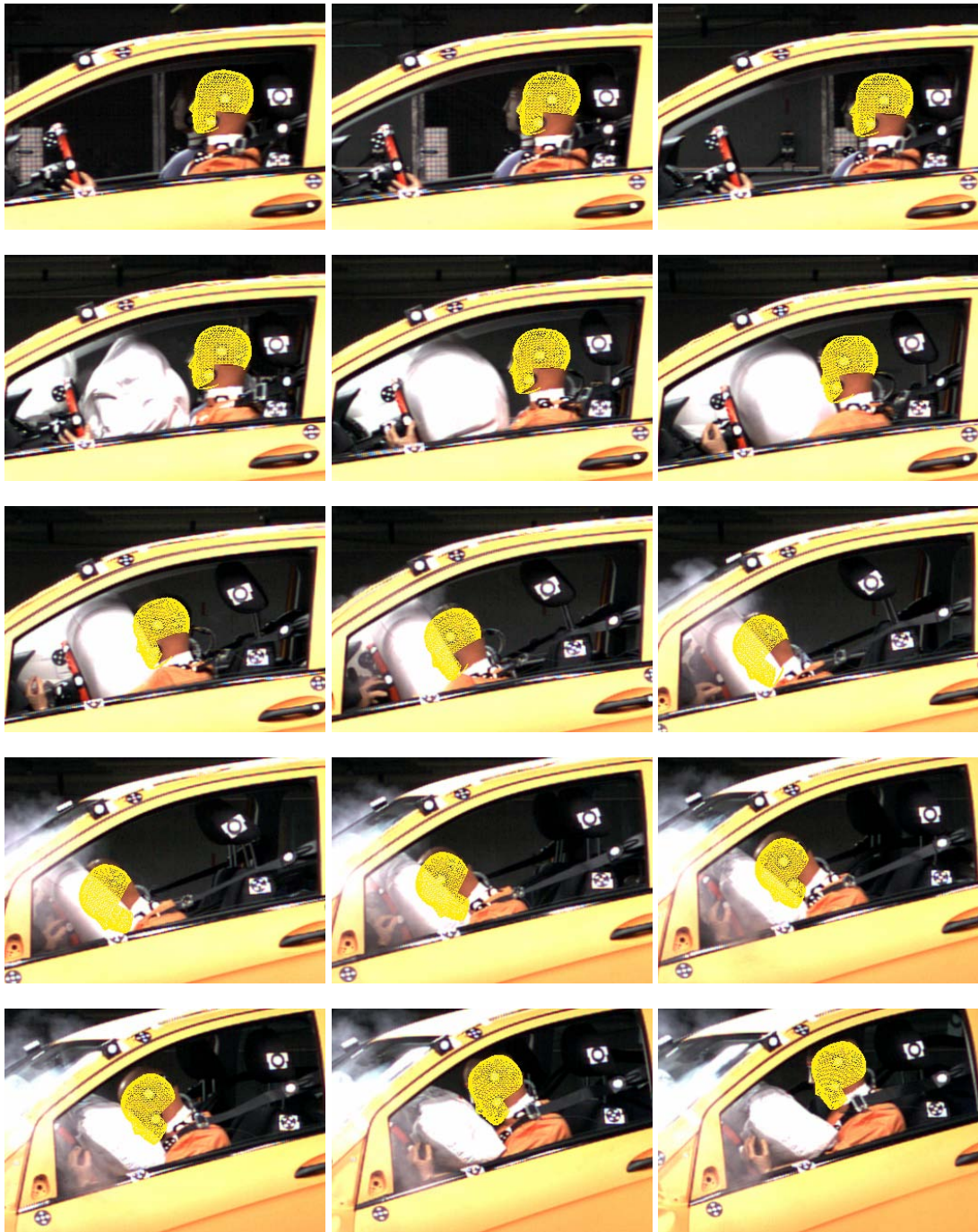
Figure 5.43: Estimated pose of the dummy's head for frames 7, 22, 37, 52, 67, 82, 97, 112, 127, 142, 157, 172, 187, 202, and 217 (from top left to bottom right).
