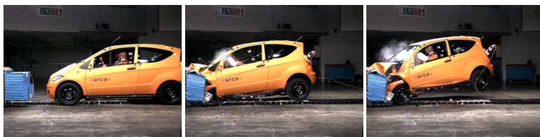
Figure 5.40: Three frames of the EuroNCAP offset crash sequence. The car jumps and moves laterally due to the offset barrier. The head is occluded by more than 50% at the moment of the deepest airbag penetration.
