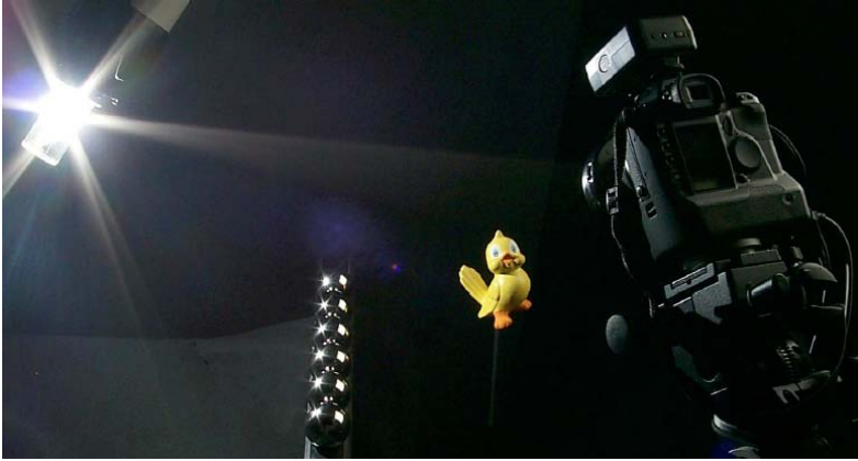
Figure 2.10: BRDF acquisition using Lensch et al. method [94]: the sampled object is illuminated with a strong quasi-punctual light source, the surface response is captured using a digital camera. Both light and camera position are calculated using the mirroring spheres
