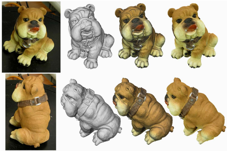
Figure 3.12: An example of color mapping. The 3D model is composed by 1 million triangles, with a mapped photographic dataset of 8 images 2560 \times 1920 . From left to right: original photos, geometry, color + lambertian shading, color only.
