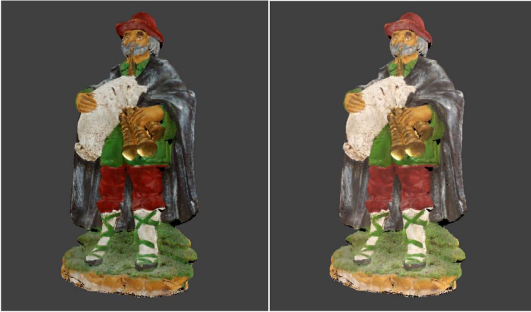
Figure 3.27: An example of color correction result, visualized with no illumination (only color values assigned to vertices); color correction is OFF in the left-most image and ON in the right-most one.
