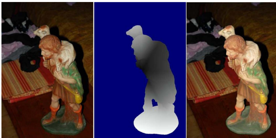
Figure 3.24: An example of color correction applied on a flash photograph: the original image (left); a normalized map of the offset correction applied to the image (center); the color-corrected image (right).
