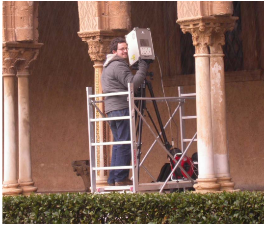
Figure 3.34: The acquisition setup adopted to scan the capitals.
