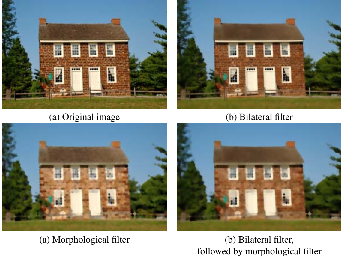
Figure 1.7: While a bilateral filter removes details based on contrast (b), a morphological filter removes details based on geometry (c). As a result, a morphological filter is able to remove highly contrasted features, but also simplifies shapes. For watercolor stylization, a combination of a bilateral filter followed by a morphological filter create large smooth color areas with few details (d)
