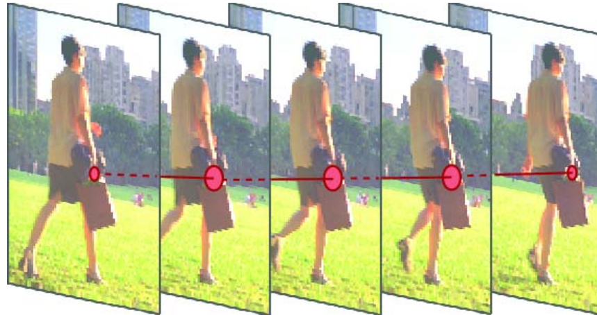
Figure 1.5: A visualization of how our tapered morphological filters follow the optical flow from frame to frame.
